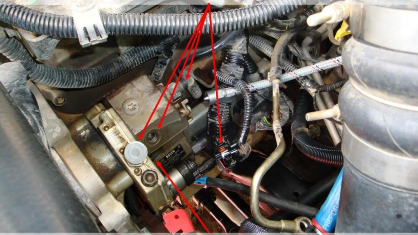
Remove the three 13mm nuts securing the CP3 to the pump mounting studs
