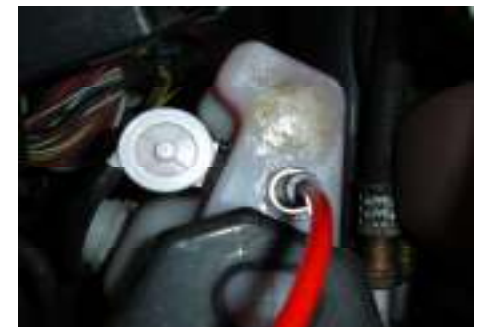
Bulkhead Fitting Installed in Washer Tank.
