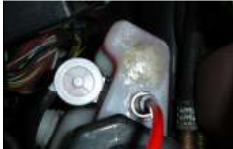
Bulkhead Fitting Installed in Washer Tank.
