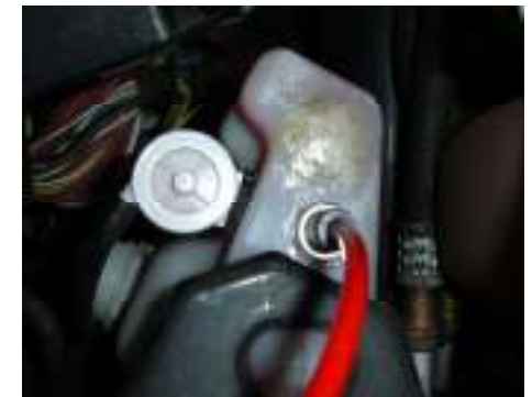
Bulkhead Fitting Installed in Washer Tank.
