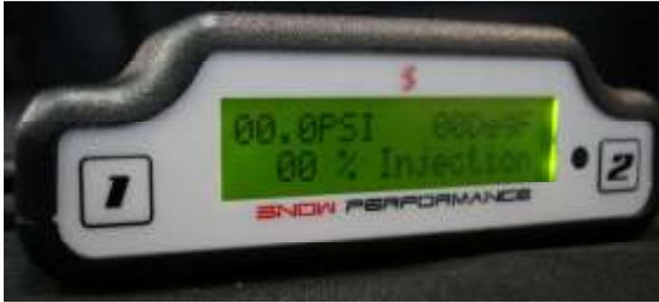
Attach controller to secure location with easy access in driver's compartment using supplied tape. Connect silicone tubing from intake plenum boost line (use the included boost 'T') to clear tubing coming from the controller and secure with a tie wrap.
