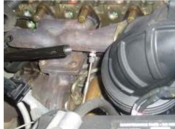
Mount the Temp Probe using the 3/16” compression fitting (provided).
