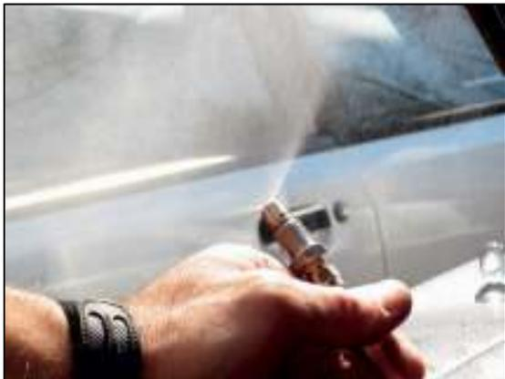
If pump goes on and fluid level doesn't go down, there is an obstruction in the tube or nozzle.
