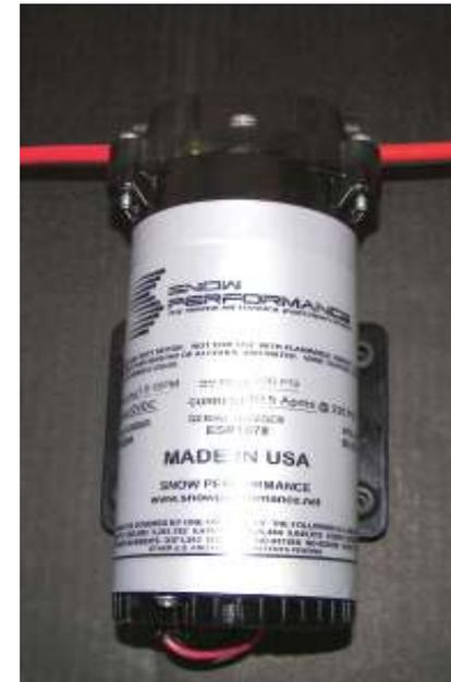
Measure the distance from the reservoir outlet to the pump inlet. Cut the ¼” red tubing using utility knife. Make cuts are as square as possible.
