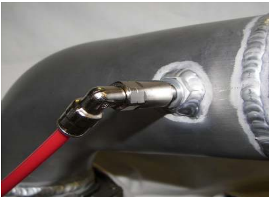
Weld-in aluminum bung shown.
