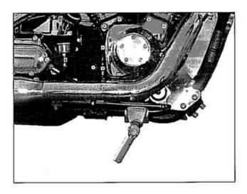
Sportster: Place bar to the front of frame. Locate base 1" to right of center of cycle to center the clamp in base. You might have to move wires to the inside of the frame tube to clear clamp, depending on model & year of cycle.
