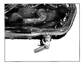
**Custom Models:** The clamping bar can be placed anywhere in which it does not interfere when the kick stand is raised.
