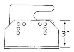
If the holes do not line up at this measurement, raise or lower the adjustable plate to the next hole. Plates will adjust at 1/4" increments only starting at 3".
