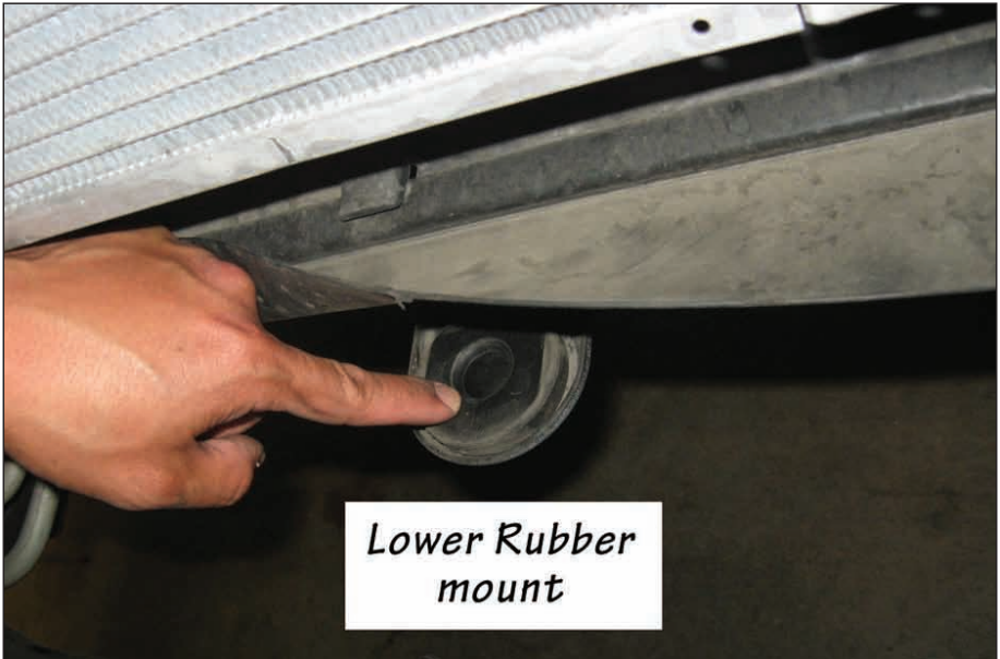
Figure 9 Connecting Fuel Cooler Radiator to Banks Techni-Cooler
