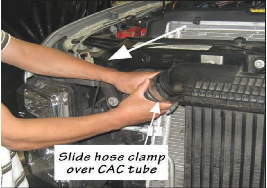
Figure 3 Disconnecting the Driver Side CAC Tube
