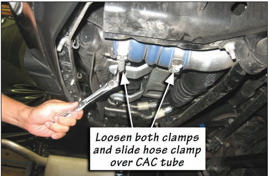
Figure 3 Disconnecting the Driver Side CAC Tube
