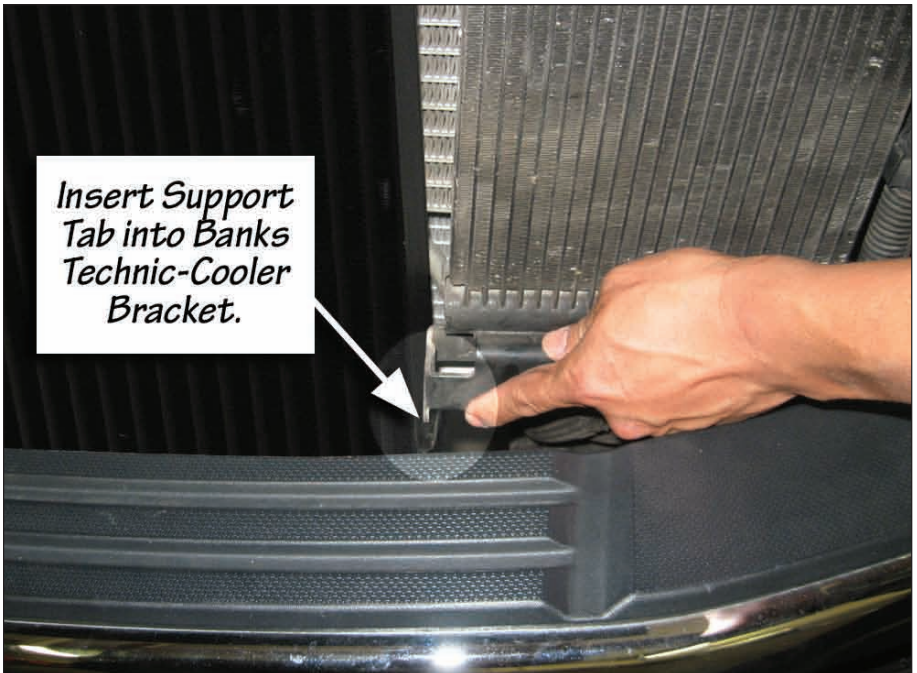
Figure 9 Connecting Fuel Cooler Radiator to Banks Techni-Cooler
