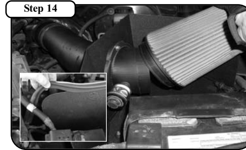
Install pre-oiled aFe filter and tighten clamp. Install trim seal on heat shield.
