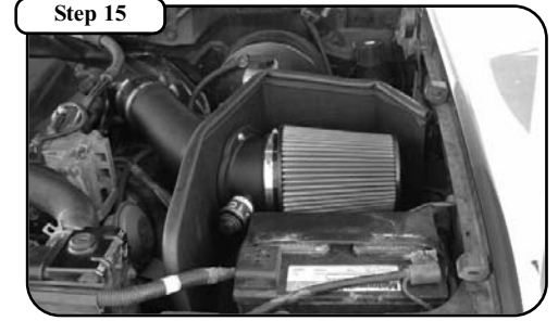
Place enclosed CARB EO sticker on a clean/smooth surface on or near the intake system. EO identification label is required in passing the Smog Check Inspection. Complete kit installed.
