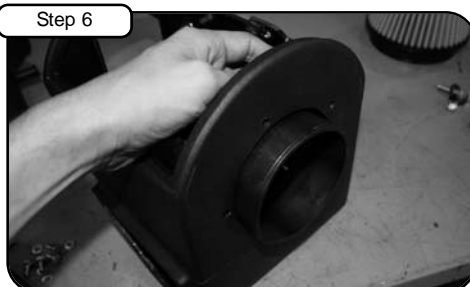
Install filter adaptor to inside of housing using button head screws and wavy washers.
