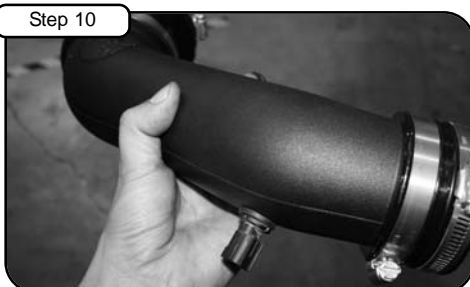
Install couplers with clamps to tube. Remove temp sensor from OE intake tube and install into new tube using grommet provided.
