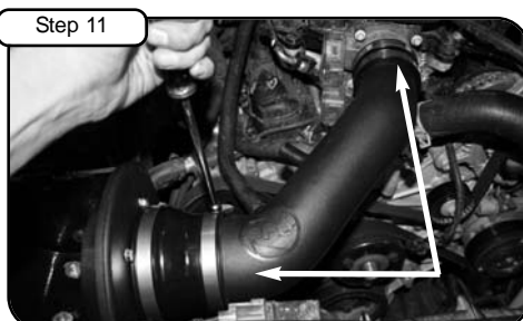
Install tube to throttle body and housing. Tighten clamps using 5/16" nut driver.
