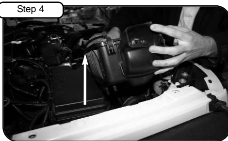
Carefully remove bottom half of airbox. (caution, this may require some force)
