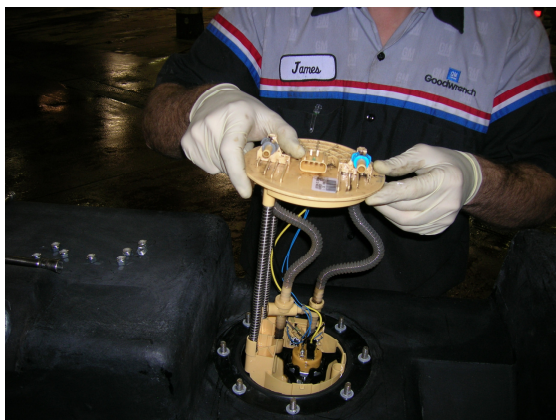
(Fig. 3) Carefully place sending unit into the TITAN™ fuel tank on top of “O” ring gasket.
