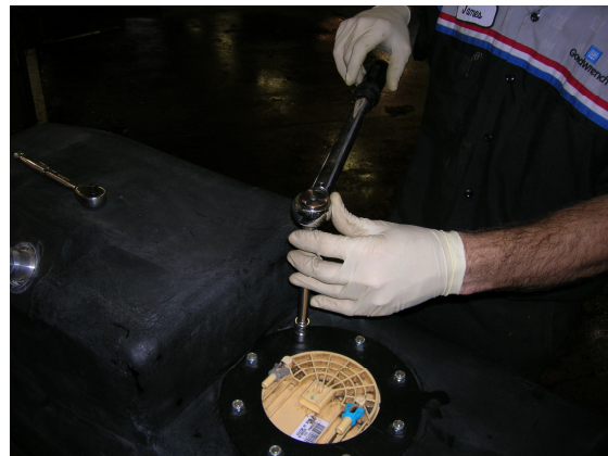
(Fig. 4) Tighten nylon locking nuts on the top flange to 20 ft. lbs of torque. Tighten in a “star” pattern.
