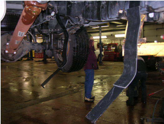
(Fig. 7) Carefully bend straps down out of the way in preparation for lifting tank into place.
