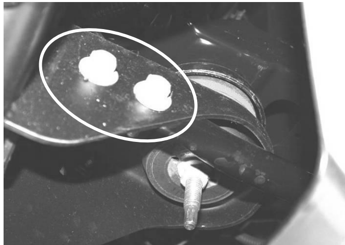
Figure 4 – Outer Bumper Support Screws
