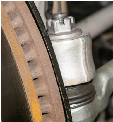
Fig. 15: Tie rod end.
