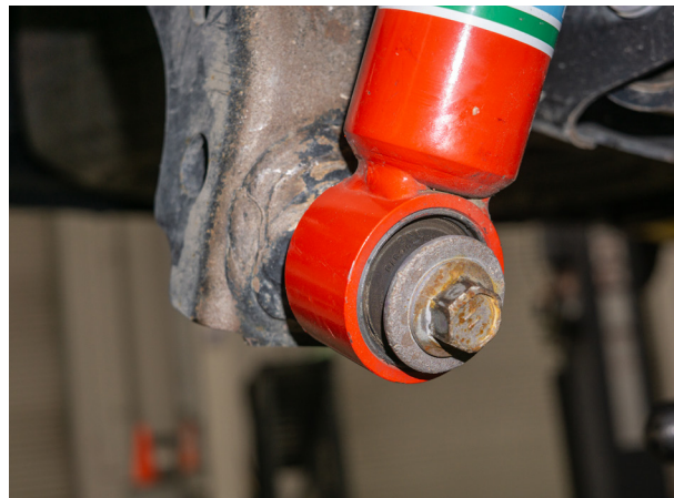
Fig. 17: Remove lower shock mount bolt.
