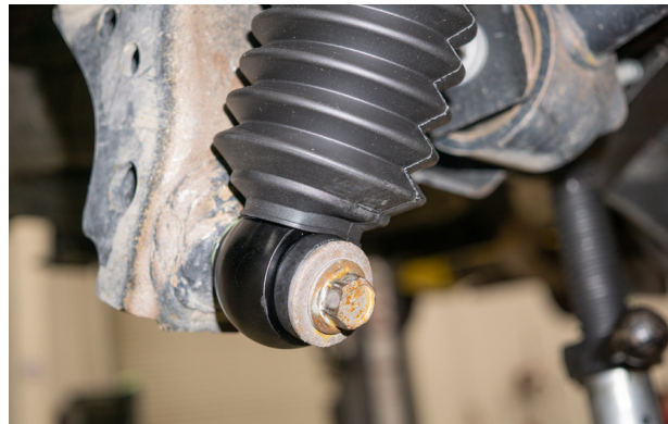
Fig. 21: Install the lower shock bolt (passenger side shown).
