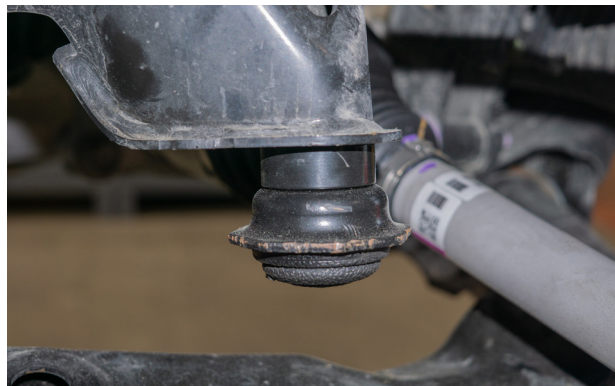
Fig. 10: Install the bump stop spacer if preload is added.
