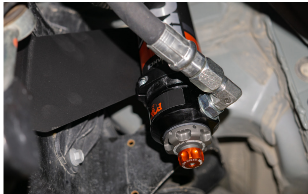
Fig. 22: Mount the reservoir to the bracket (driver side shown).
