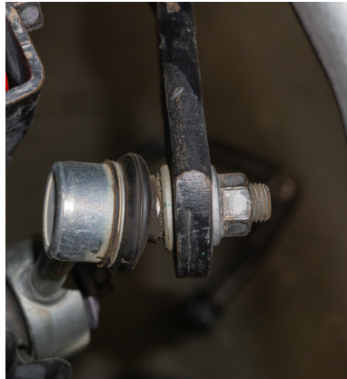
Fig. 16: Sway bar end link.
