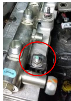
Figure 13A: 10MM bolt retaining the grid heater power supply harness on intake plenum.
