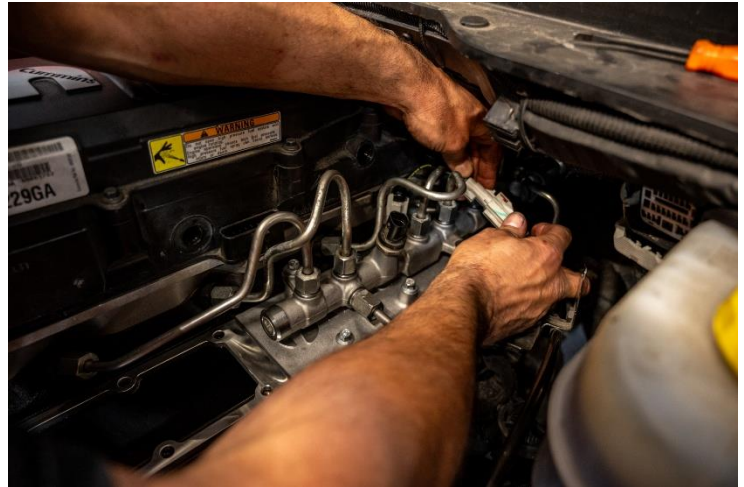
Figure 25: Rail pressure sensor and charge air harness.
