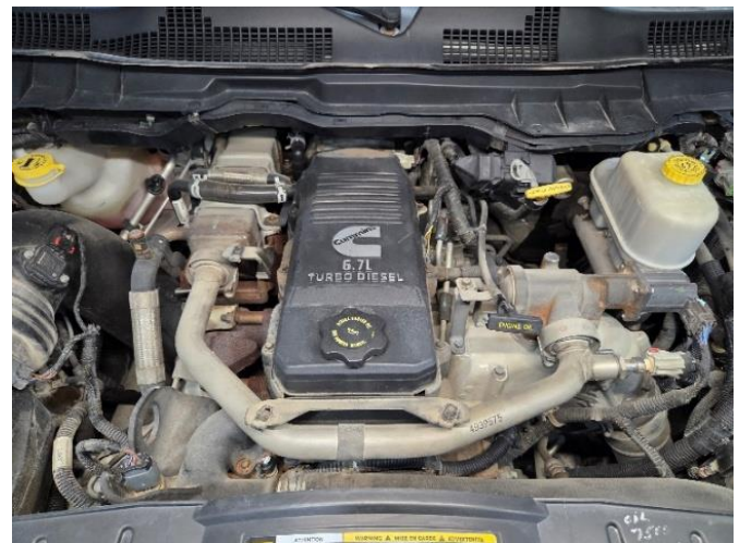
Figure 43: EGR Crossover tube reinstalled Model Years 2013-2018.
