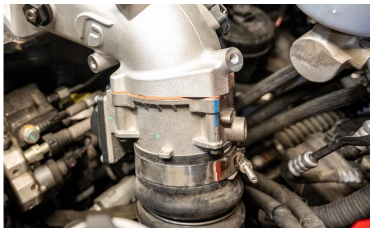
Figure 35: Throttle valve with CAC Boot attached.
