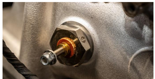
Figure 38: New heater with included M5 nut, used to retain new heater harness.
