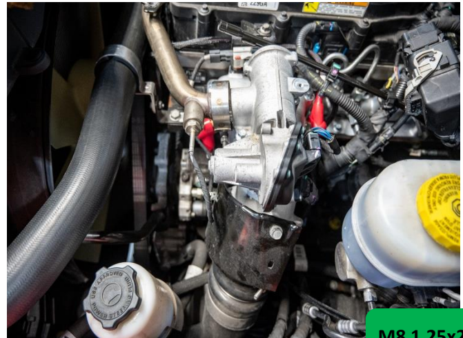
Figure 42: EGR Valve reinstalled, M8 1.25x25 bolts hand tight.
