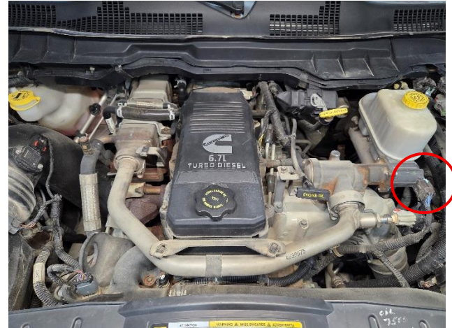
Figure 7: Engine cover removed. EGR control valve connector is circled. The EGR temperature sensor is pictured off to the left of it.
