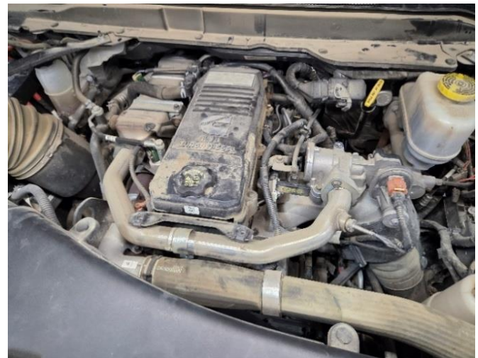
Figure 44: EGR Crossover tube reinstalled Model Years 2019-2024
