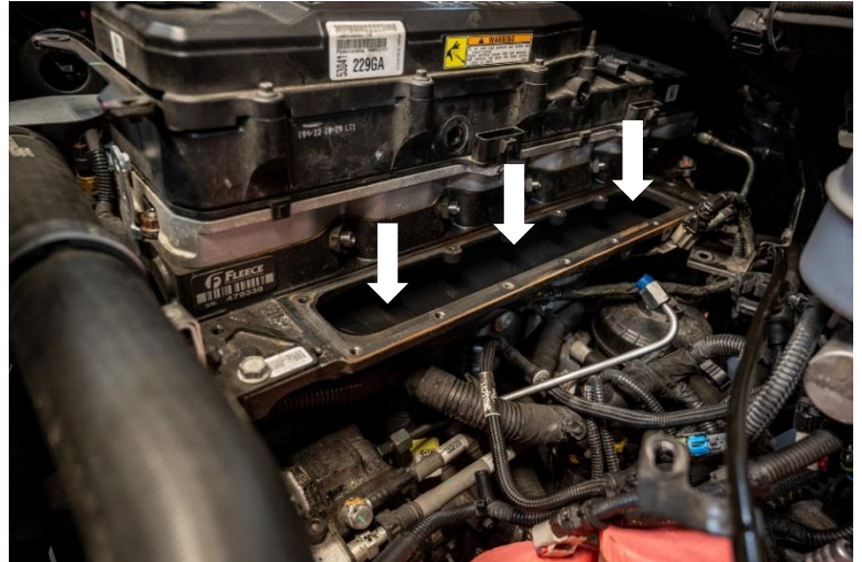
Figure 18: Intake plenum and gasket fully removed
