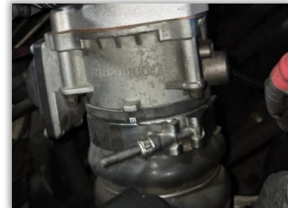
Figure 13B: Throttle valve with CAC boot attached.
