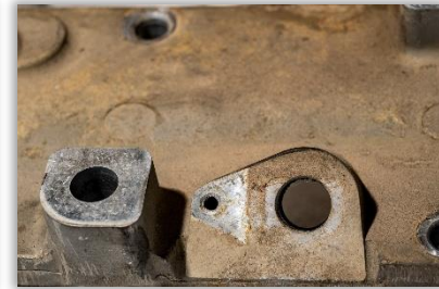
Figure 8B: MAP sensor Location on intake plenum.
