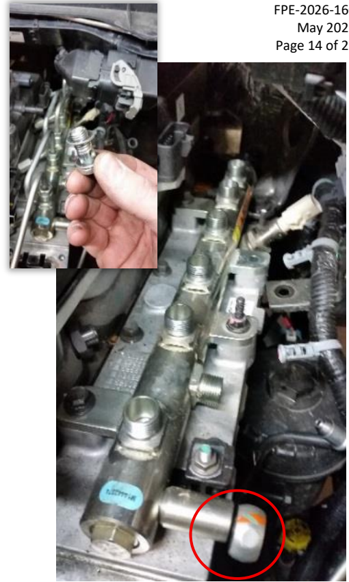
Figure 16: Injection lines removed, fuel return line circled.
