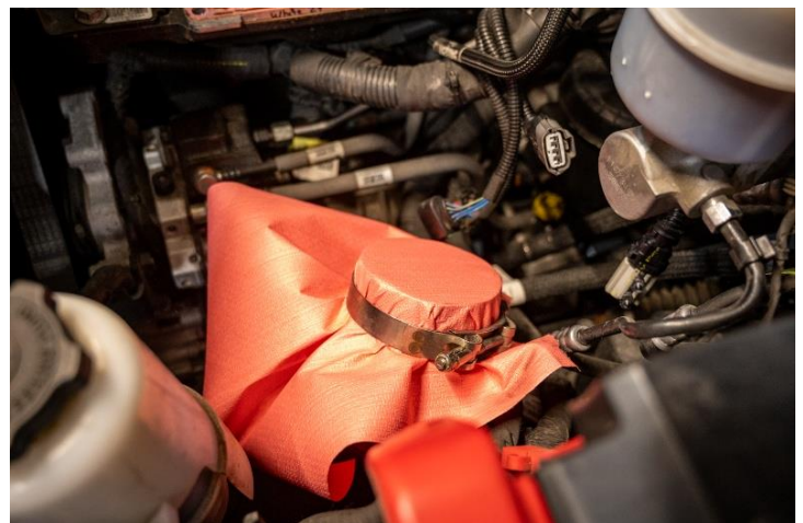
Figure 10: CAC boot covered with shop towel; clamp placed over top to secure.
