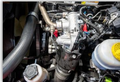
Figure 13A: Shroud over top of CAC boot.
