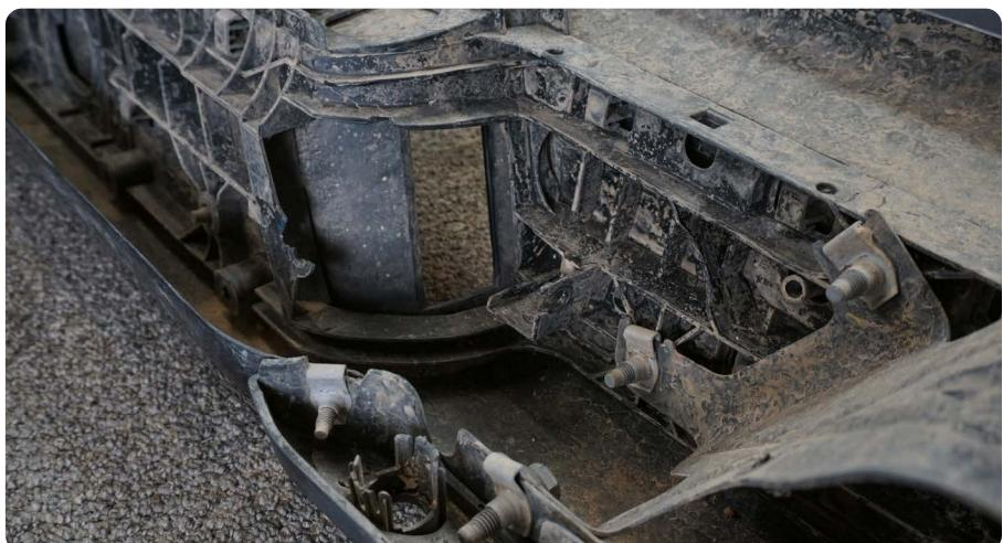
**STEP 11 |** Begin by installing the trailer plug socket into the DV8 rear bumper. Press firmly until the socket is fully clicked into place.
