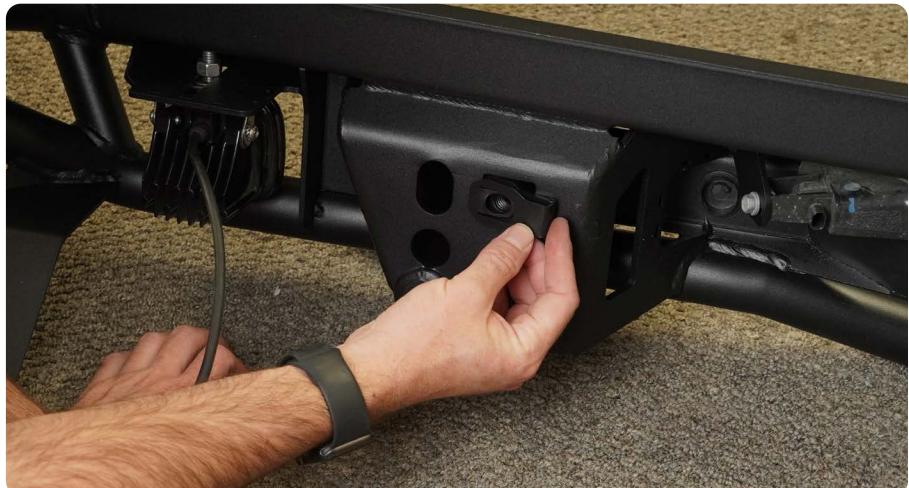
**STEP 15** | Mount your license plate to the bumper using the provided M6 allen head hardware, a #4 allen tool and a 10mm socket or wrench.
