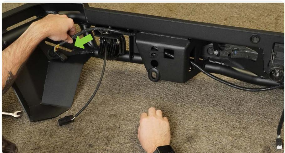
**STEP 18** | Use the built in zip-tie tabs to secure the wiring harness to the bumper.
