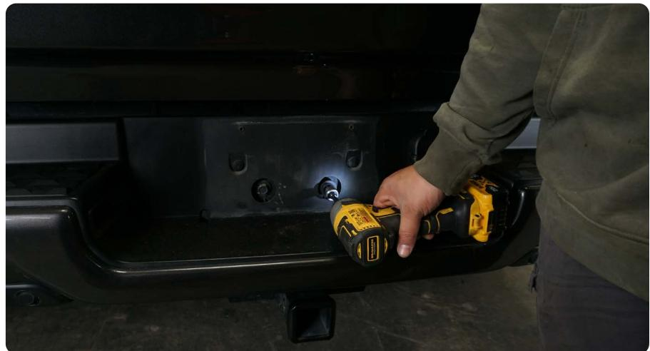
**STEP 5 |** Using a 16mm socket or wrench, remove the (4) nuts (2 per side) to release the bumper.
