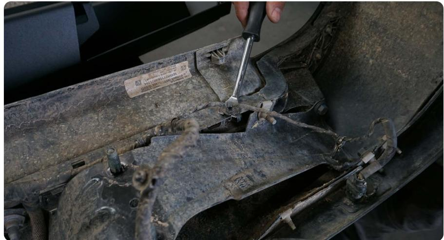
**STEP 7** | Once the wire harness is free from the bumper, disconnect the two license plate lights by depressing the tab on the plug and pulling away from the light.
