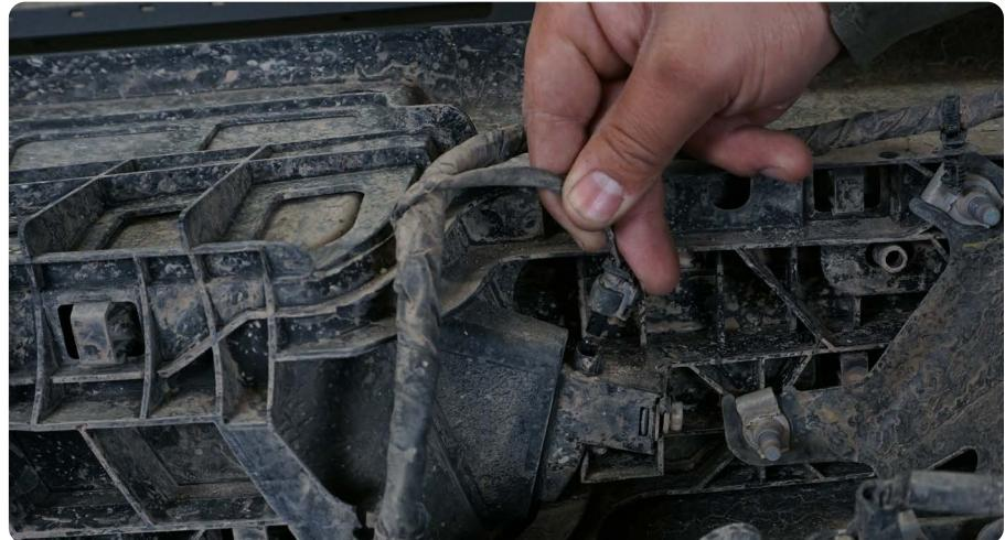
**STEP 8** | Next, remove the sensors (if equipped). Do not unplug the sensors, rather, gently spread the two clips on each side of the sensor and pull the sensor back away from the bumper.
