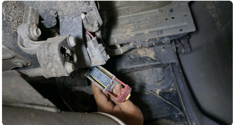
**STEP 3** | Disconnect the wiring from frame releasing a trim clip tool so that the wiring is free.
