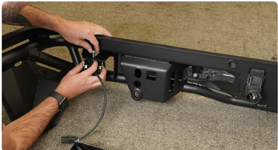
**STEP 14** | Install the provided nut clips onto the bumpers mounting points. (1 nut clip per side).
