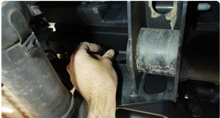
**STEP 23** | Double check the height of the bumper to ensure the bumper is not rested on the dual exhaust tips (if equipped).
