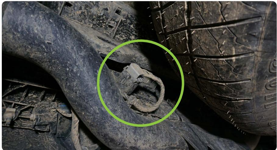
**STEP 2** | Above the exhaust (on a dual exhaust vehicle) remove the large connector for the rear bumper. This is held on by a push pin. Flip up the latch, and the plug should disconnect itself.
