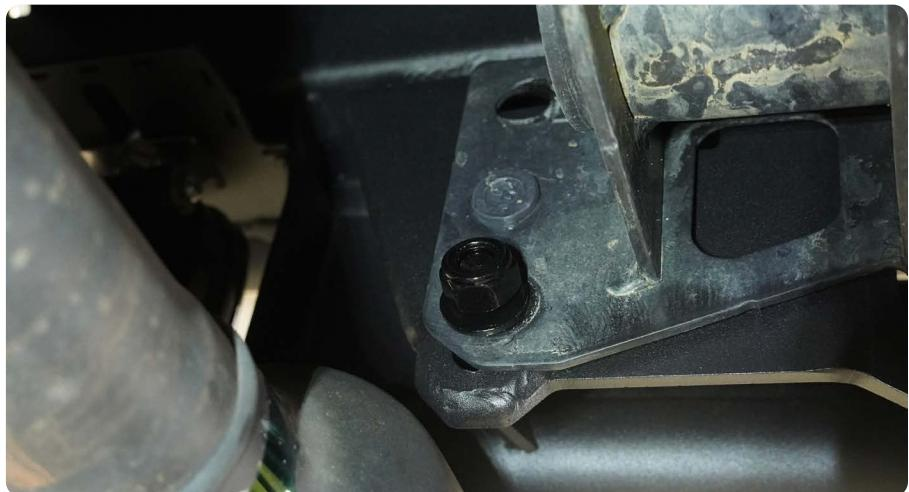
**STEP 22** | Use the provided M12 hex head bolts and a 17mm wrench or socket to loosely secure the top of the bumper using the previously installed M12 nut clip.
