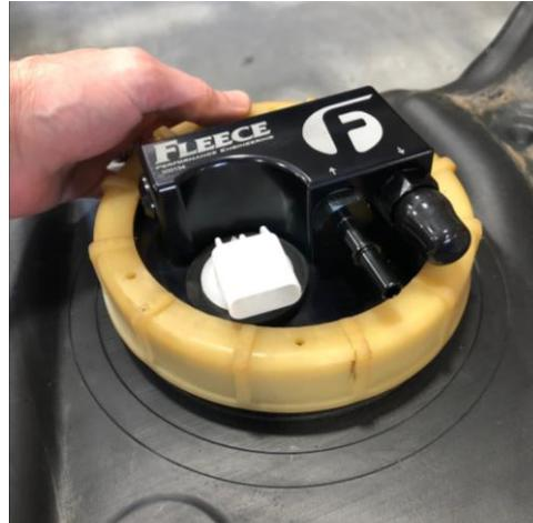
*NOTE: Use caution when installing the SureFlo to not damage the float arm. DO NOT rotate it once installed in the tank, you may damage the float arm or sending unit – align the pump before you place it into the tank.*
