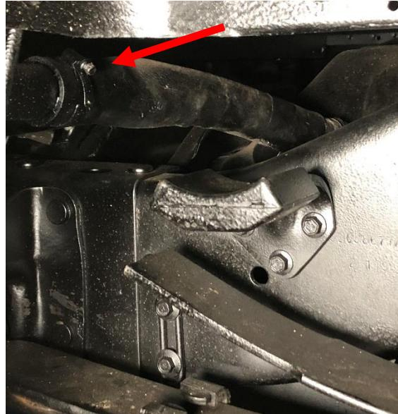
STEP 2: Reaching over the top side of the tank, disconnect the fuel lines and electrical connection for the OEM sending unit.
