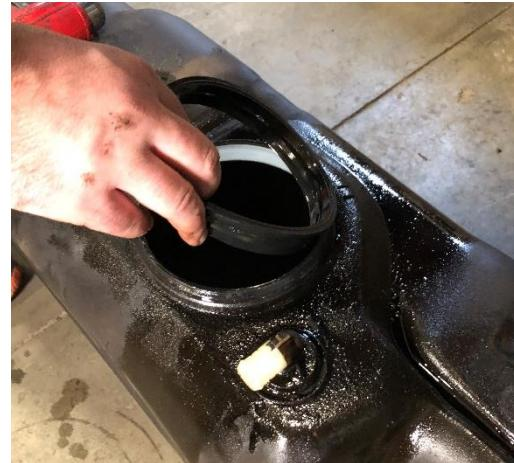
STEP 9: Install the new gasket included in the kit into the fuel tank. Clean the original retaining ring of debris and prepare it for re-use onto the new SureFlo sending unit.
