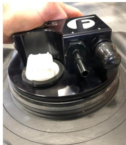
STEP 12: Reinstall the retaining ring using your hammer and punch or a strap wrench by rotating it clockwise to the fully engaged position
