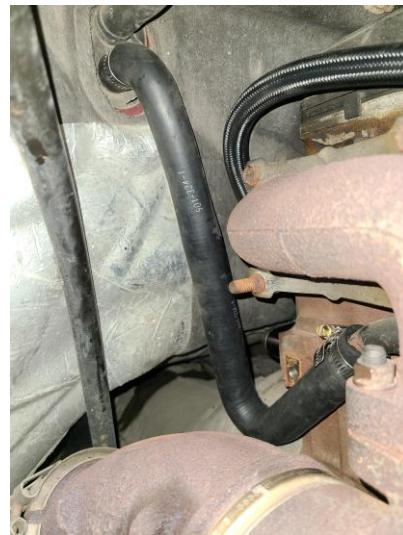
**STEP 8:** Using an 8mm Socket, remove the three bolts anchoring the stock thermostat housing. It is not necessary to remove or disconnect the thermostat housing from the upper radiator hose. Move it to the side, out of the way of the exposed thermostat, to allow for access.
