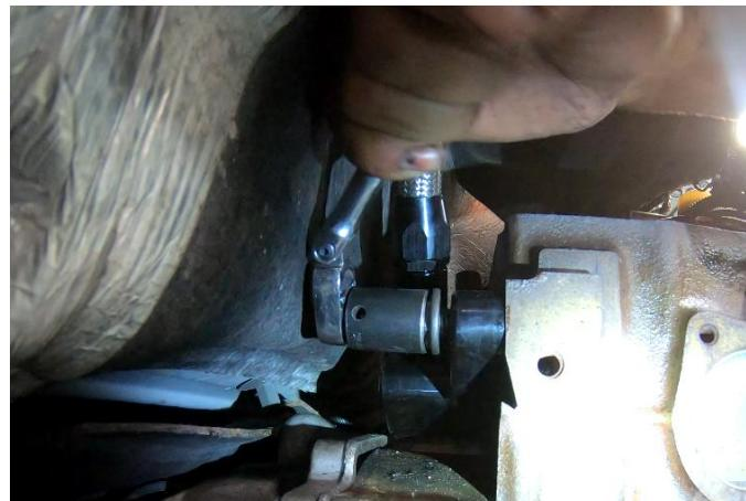
**STEP 18:** With the coolant line routed above the exhaust manifold, thread the available end onto the AN style fitting of the installed thermostat riser block.
