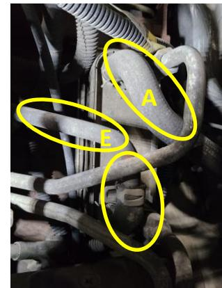
**STEP 4:** Remove the hose from the transmission heat exchanger that runs to the side of the engine block (section E). Remove the threaded barb fitting from the engine block.
