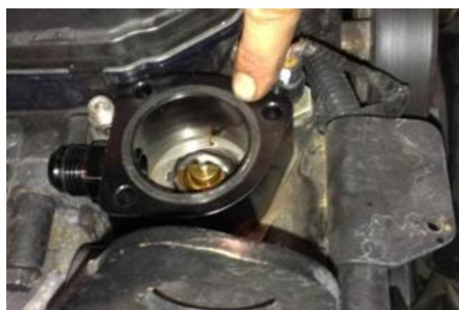
**STEP 11:** Place the stock thermostat housing over the thermostat riser block. Using the supplied M6 flange head bolts, tighten the bolts to 89 in-lbs.
