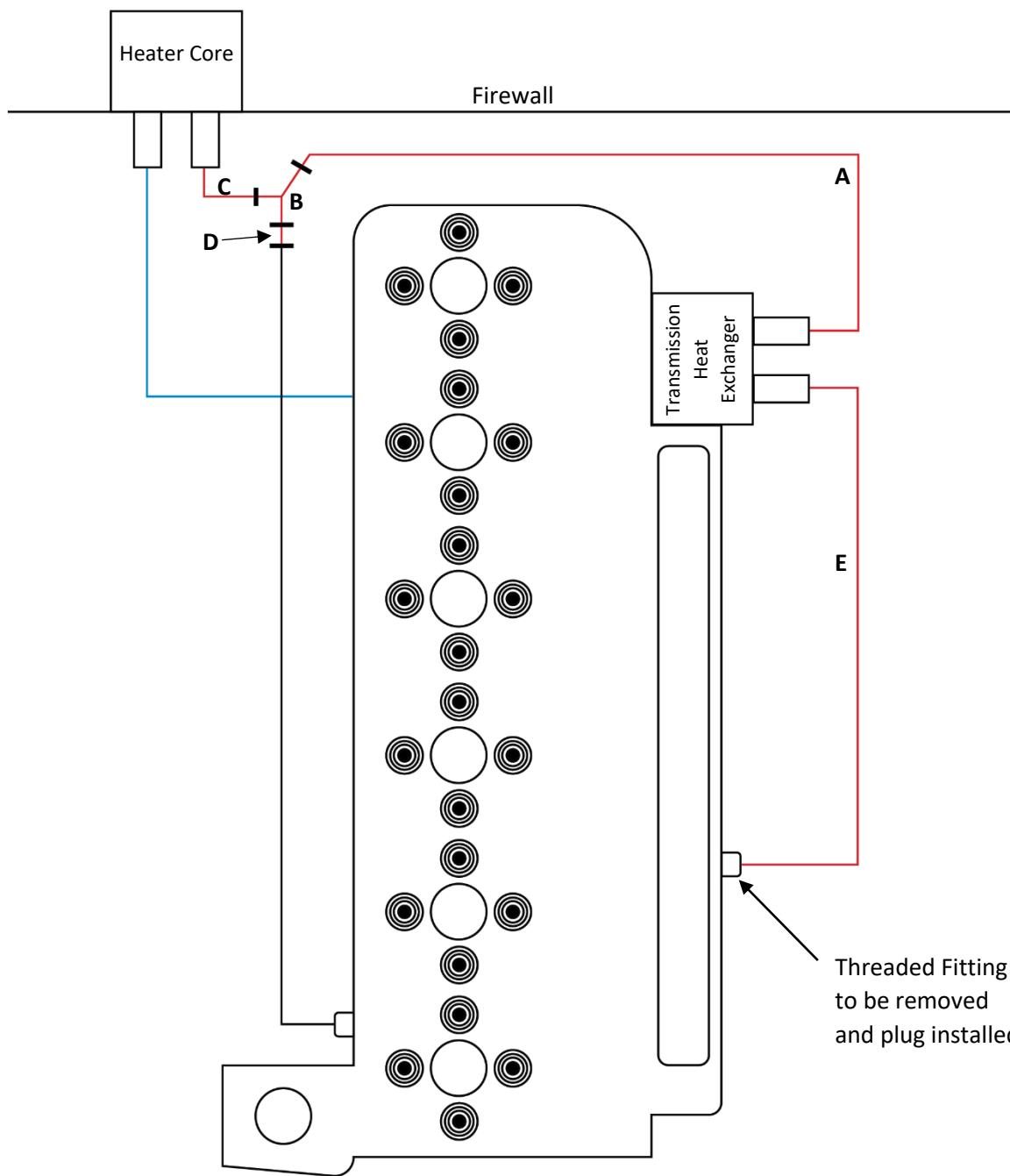
**STEP 5:** Install the rubber caps onto the open ports on the transmission heat exchanger.
