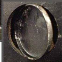
**STEP 13:** With the freeze plug removed, use a Scotch-Brite™ pad and a degreasing solution to **thoroughly** clean the block surface area from the head down to the rear cover, as well as the bore where the freeze plug was previously installed. Be sure to remove all dirt and foreign debris to allow the coolant bypass thermostat housing to fully seat.
