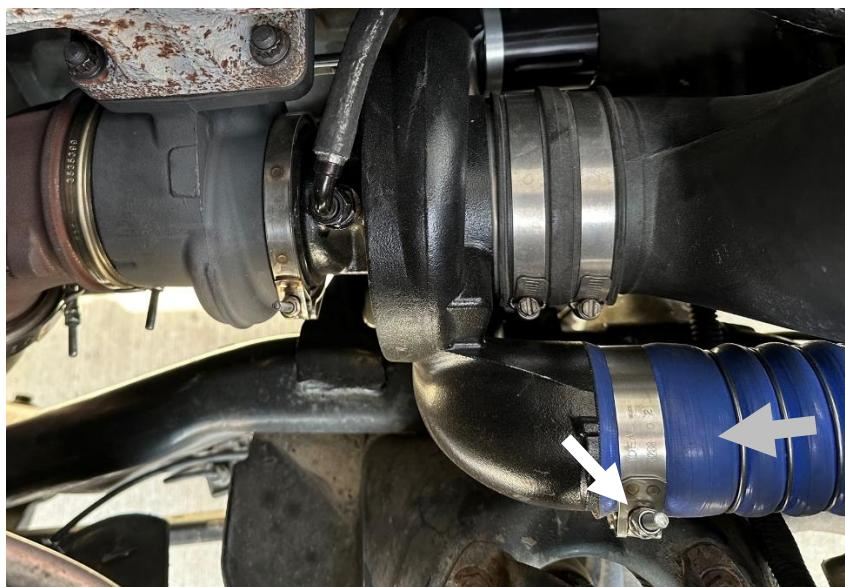
8. Connect the exhaust elbow to the turbocharger and tighten the clamp bolts to 11 N·m (100 in. lbs.) torque.
