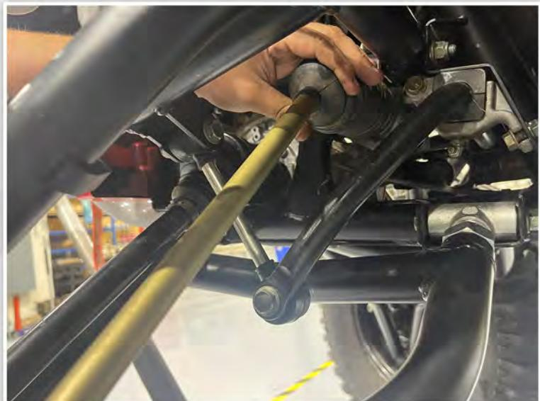
NEXT, LOOSEN THE INNER TIE ROD END FROM THE RACK.
