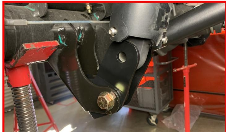
Assemble the 14" straight end links (Add rubber bushing to the end link then add crush sleeve to the bushing.)
