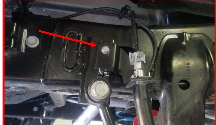
Remove the rear **wheel speed** sensor and **brake caliper**, **WARNING**: Use a hanger to support the caliper, don't let it hang from the brake line or the ABS wire.
