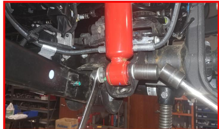
Remove the **front track bar hardware** at the axle. Be sure to retain factory hardware.
