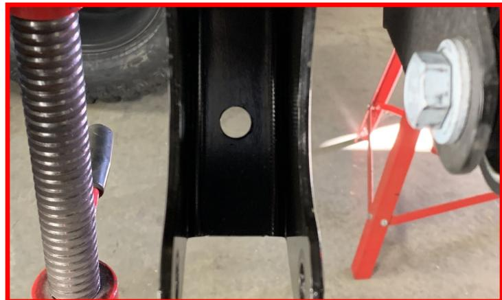
Install the supplied rear shock extension Using the supplied **M14 x 70mm bolts, washers and nut and the supplied M12 x 30mm bolt, M12 washer and nuts** through the shock extension and axle mount.
