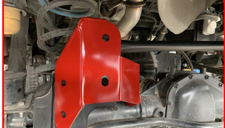
With the **track bar relocation bracket** on the factory axle mount, mark the (2) 1/2" holes located on the back of the bracket.
