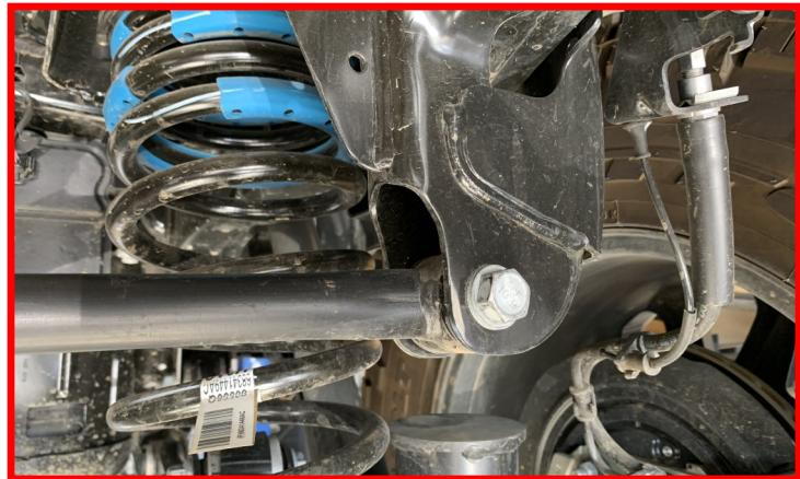
Loosen the **track bar mounting bolt** at the axle.
