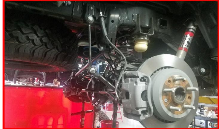
Remove the **rear brake line bracket** at the frame rail.
