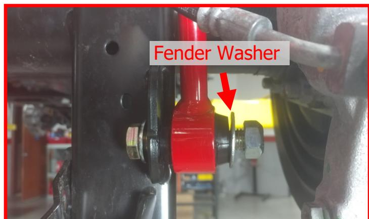
Attach the ReadyLIFT brake line bracket to OE bracket using the provided **1/4" x .75" bolt, washers and nut**. Gently rotate/bend the metal brake line. Install using the **factory hardware**. Torque all to **5 ft-lbs**.
