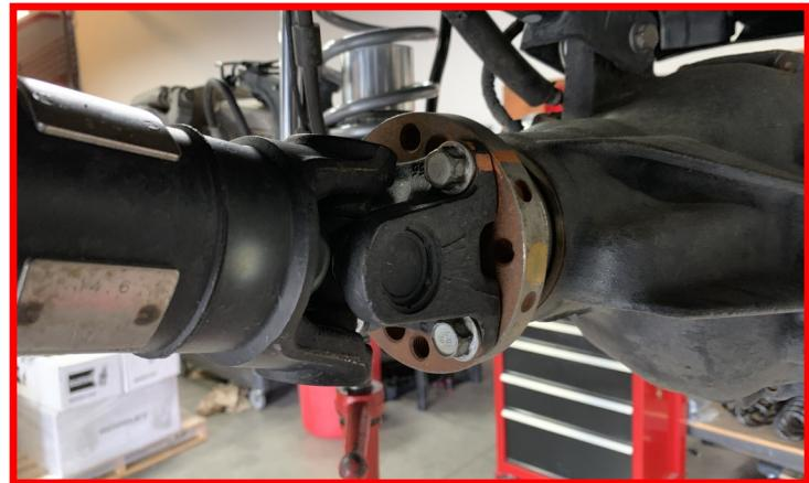
Install the wheels and lower the vehicle to the ground. Torque the lug nuts to the wheel manufacturer specs. Jounce the vehicle a few times to settle the suspension to the new ride height. Torque the upper control arms to **110 ft-lbs**, lower control arms and track bar hardware to **135 ft-lbs**, shock hardware to **90 ft-lbs** and sway bar end link hardware to **50 ft-lbs**. Reinstall the upper control arm heat shields. Torque to **5 ft-lbs**.
