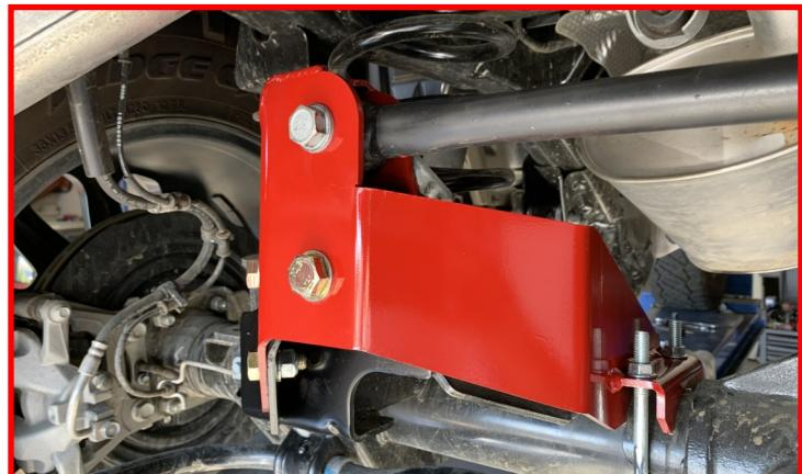
Remove the lower control arms and discard retain factory hardware. Install the **replacement lower control arms** with the bend facing inboard and the shorter . Do not tighten at this time.
