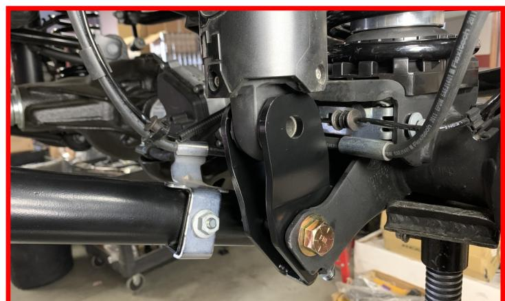
Install the factory shock into the shock extension using the factory hardware.
