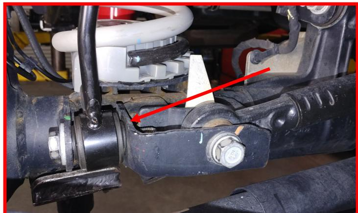
Remove the front sway bar end link from the sway bar. Discard as it will not be re-used.
