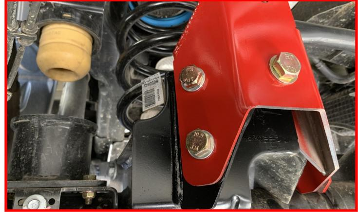
Tighten the U-bolt hardware.
