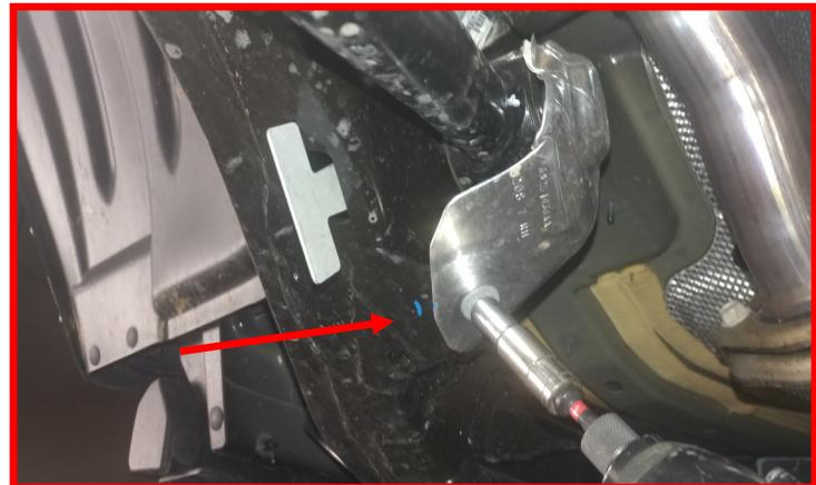
Gently pry the heat shield out of the way and loosen but do not remove the **front upper control arm bolts**.
