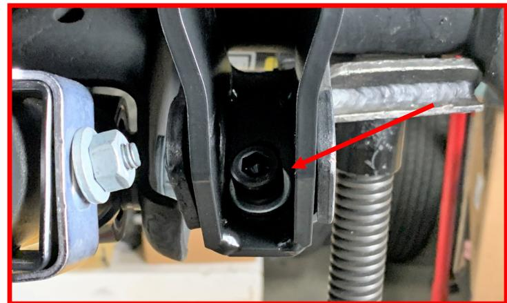
Once the **M12 shallow socket head allen bolt, M12 washer and nuts** have been installed and torqued. Install the **front shock extension crush sleeving**.
