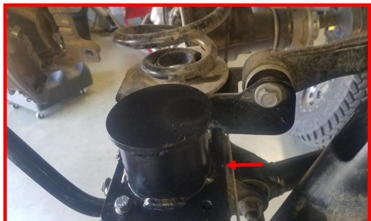
Remove the **track bar mounting bolt** from the axle mount.
