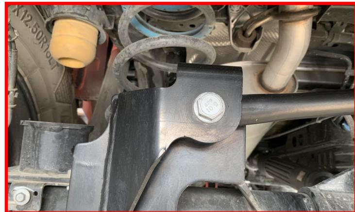
Lower the axle enough to remove the stock spring and rubber isolator. Discard the factory springs at this time.
