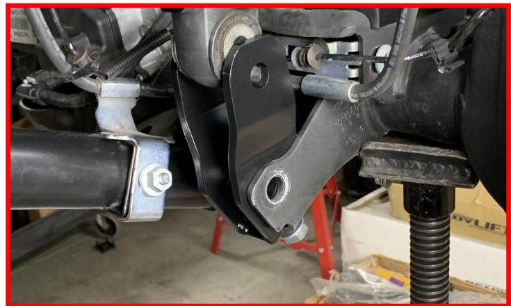
Install the supplied **M12 shallow socket head allen bolt, M12 washer and nuts** through the shock extension and axle mount.
