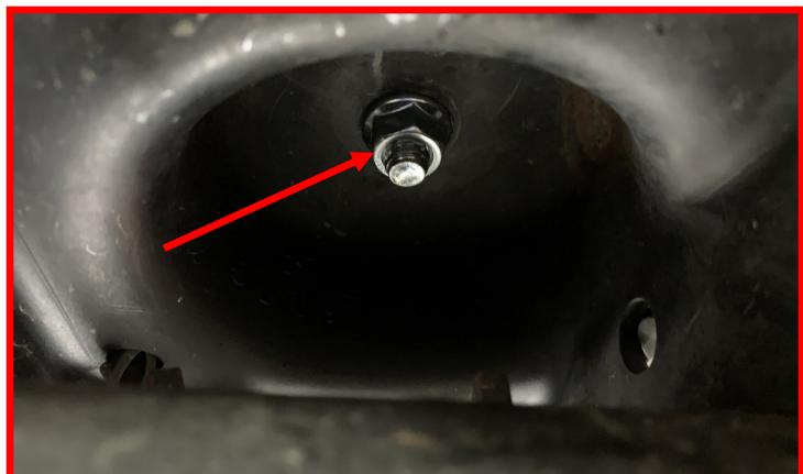
Using a **1/2"** drill bit, enlarger the existing hole on the front axle shock mounts.
