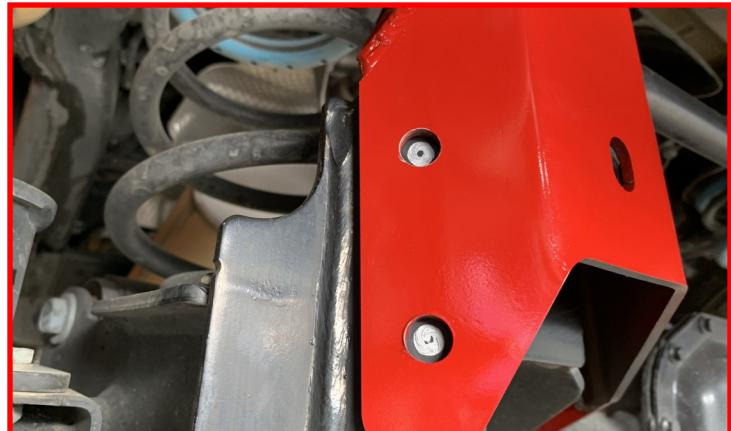
Remove the **track bar relocation bracket** from the factory axle mount.
