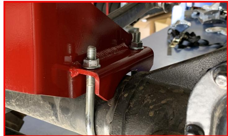
Tighten both the M14 and M12 hardware at this time.
