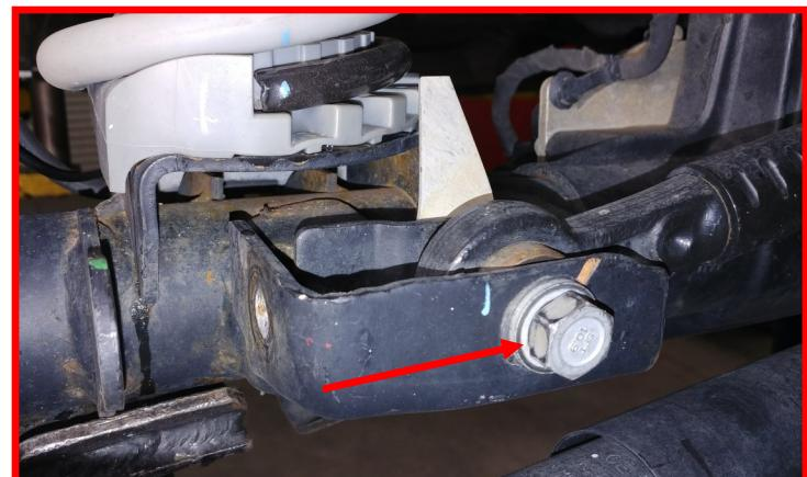
Remove the **front track bar bolt** at the frame. Retain factory hardware. Remove complete track bar assembly from vehicle and discard.
