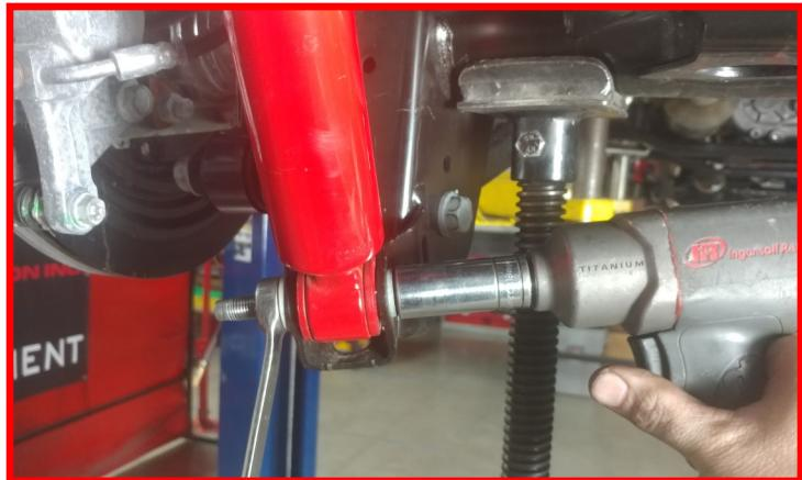
Remove the rear sway bar end link from the axle and sway bar and discard, retain the factory upper hardware.
