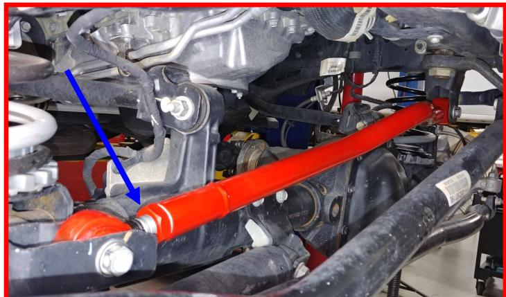
With track bar installed be sure to verify the rod end **jam nut** is tight.
