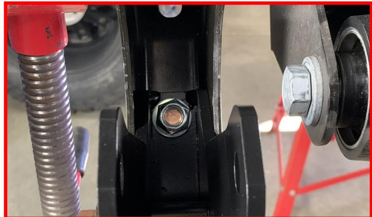
Install the factory shock into the shock extension using the factory hardware.
