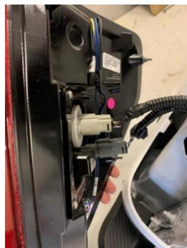
5. If your 52900XX wire harness ends in 12, 17, or 39, you must also install a wire harness that pulls reverse signal from the 7-pin trailer connector.
