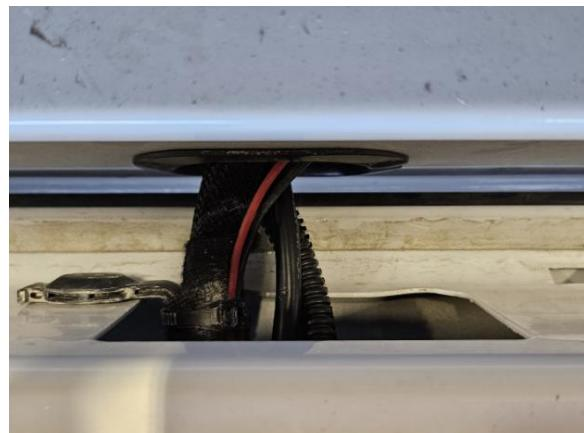
25. Connect the plug and play 4-pin connector and the light bars 4-pin connector as well as the weatherpack connectors.
