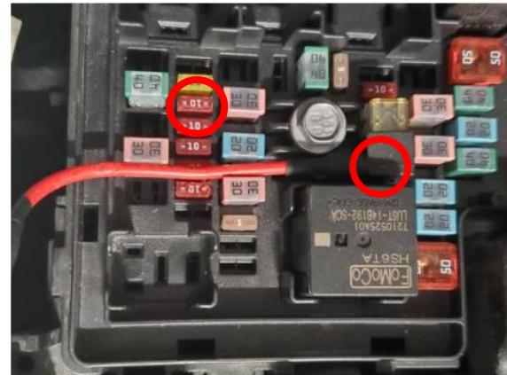
30. The fuse you take out of the fuse box goes into the bottom slot of the ACC connector. Reinstall the fuse box cover.
