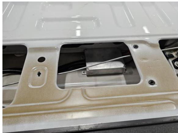
22. Connect the light bar to the driver box. Make sure the pins align, do not force the connectors.
