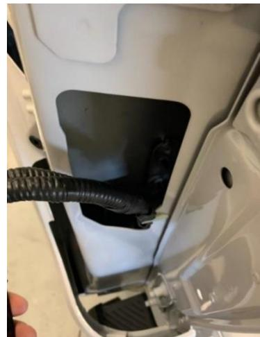
4. Disconnect the factory harness from the taillight. Now plug the female end of the in the Putco quick disconnect harness into the tail lamp and the male harness into the factory harness. Repeat on the other side. Reattach the taillights to the truck.
