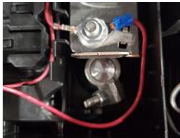
29. Connect the ACC wire to a fuse circuit which is on when the truck turns on, and is off when the truck turns off, such as 101- L headlight or 21- headlamp run/start feed depending on trim level.
