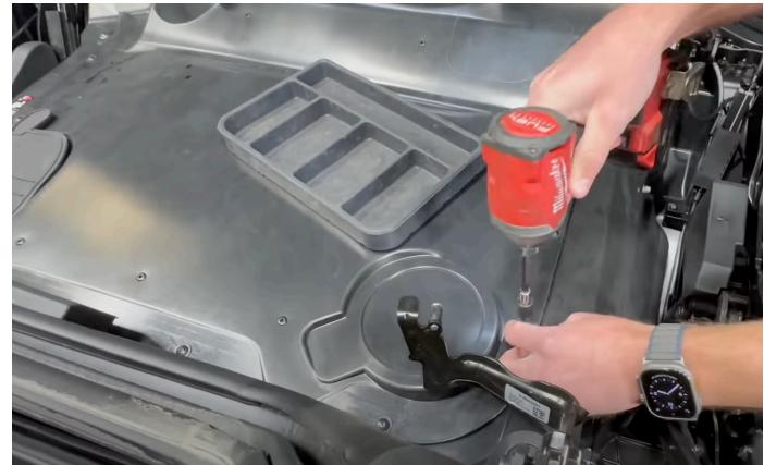
Remove the 10mm bolt and slide the coolant tank out of the way.
