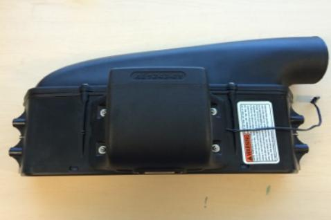
2. Remove all four screws and remove the fan exhaust with a 2.5mm hex key.
