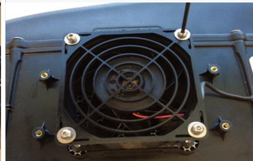
8. Reinstall the fan exhaust and tighten the four screws. Be careful not to over tighten.
