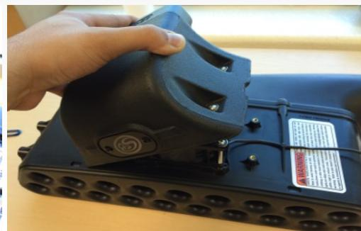
3. Remove the four screws securing the scavenge fan to the housing. Remove the fan. Note where the fan harness is located and how the fan is sitting on the housing. The fan guard is installed on the exhaust side of the fan. **Do not remove the fan guard.** Removal of the fan guard will not increase the performance of the Particle Separator and could result in serious injuries. The fan must be reinstalled the same way it was disassembled.
