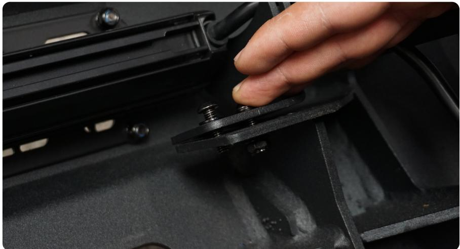
**STEP 20 |** If planning to run a winch, install your chosen fair-lead and winch at this time.
