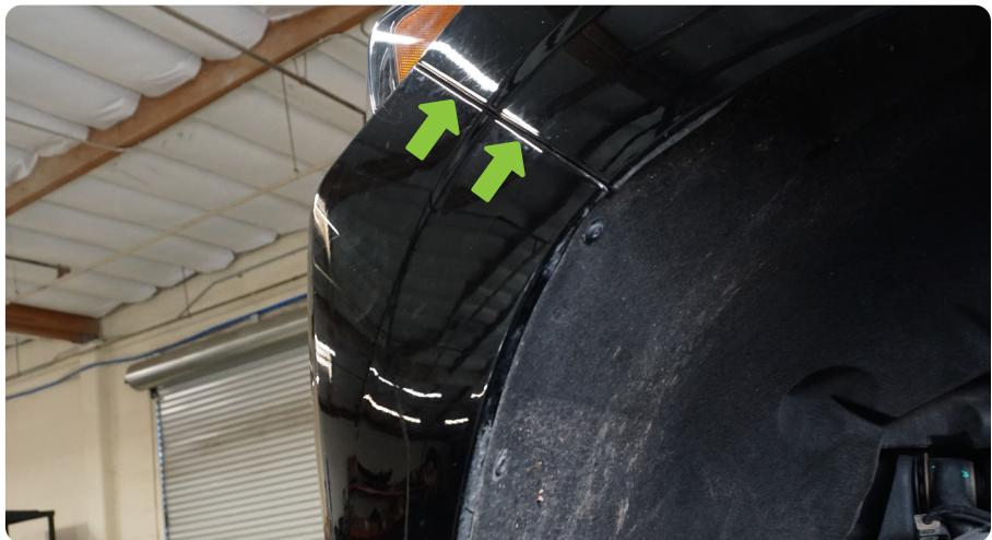
**STEP 47** | Use a T15 torx tool to secure the inner fender to the bumper/grille assembly.
