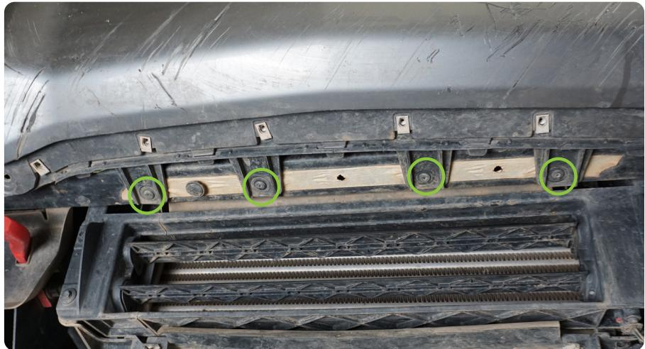
**STEP 7** | Start to pull the bumper/grille assembly away from the vehicle. If equipped disconnect the fog lights and front camera harnesses on the passenger side.
