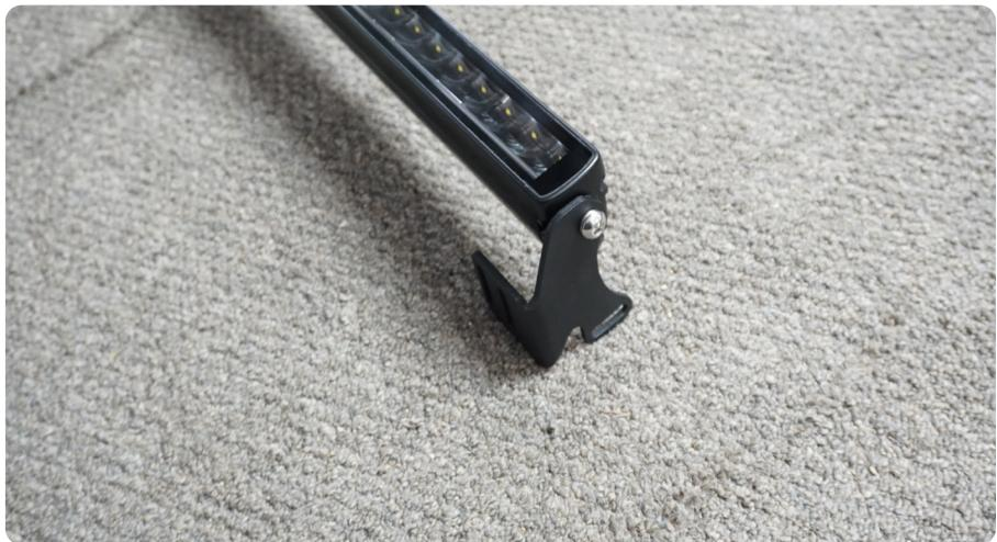
**STEP 19 |** Use the provided M6 hardware to mount the light bar brackets. Use an #4 Allen tool and 10mm wrench to secure the brackets.
