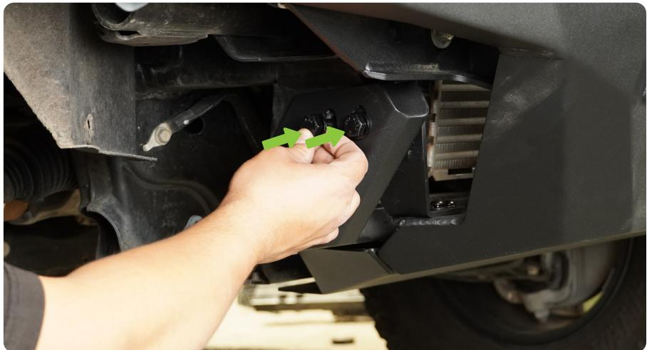
**STEP 37** | Using a 18mm and 19mm socket or wrench, secure the M12 bolts.
