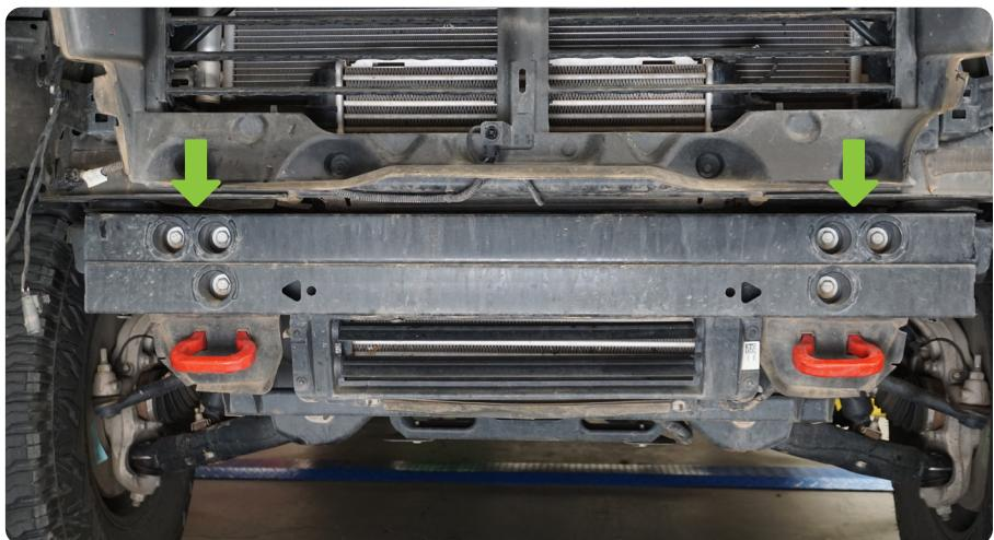
**STEP 9** | Use a 10mm socket to remove the (4) bolts that secure the lower air shutter.
