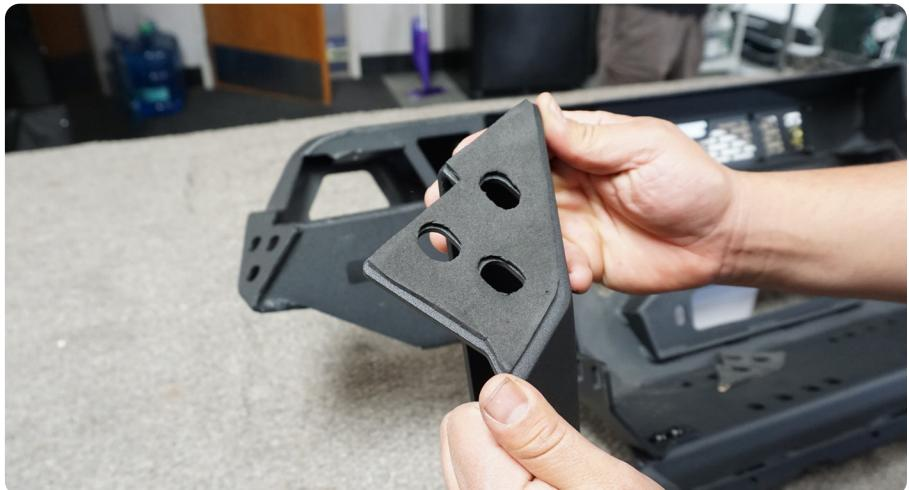
**STEP 17** | Loosely attach the bumper wings onto the bumper using the provided M10 hardware, an 18mm socket and an 19mm wrench.
