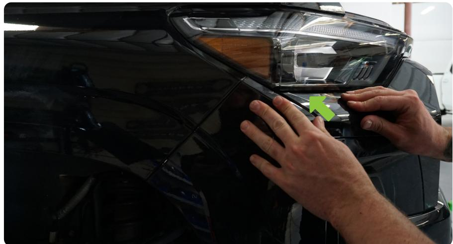
**STEP 45** | Check that the cut is even across the bumper. Additional trimming may be required.
