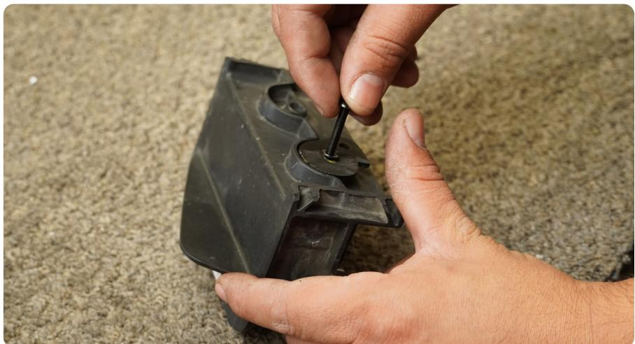
**STEP 31** | with the bolt inserted, press on the backside to score the housing and using the 3/16": drill bit, carefully drill though to allow the bolt to be through bolted.
