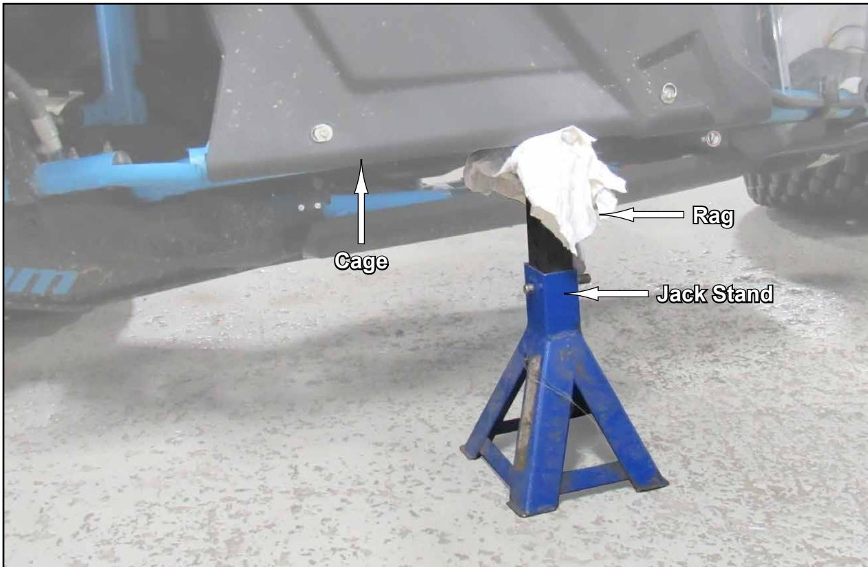
remove stock Skid Plates and hardware
