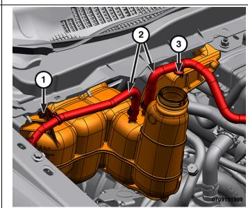
12. Cut the cable ties (1, 2) securing the NOx sensor wire harness, actuator harness, and turbo speed sensor harness.
