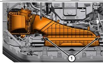
29. Install the air cleaner hose (2), and tighten the hose clamps to **11 Nm (8 ft-lbs)**.
