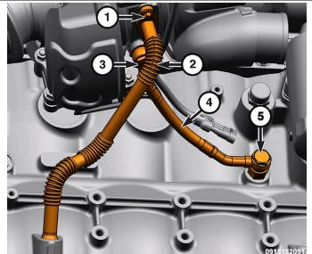
22. Remove the bolts (1, 3) securing the transmission oil cooler line bracket and the exhaust isolator (2) to the transmission.
