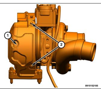
29. Remove the turbocharger speed sensor (2), and set it aside to reuse later.
