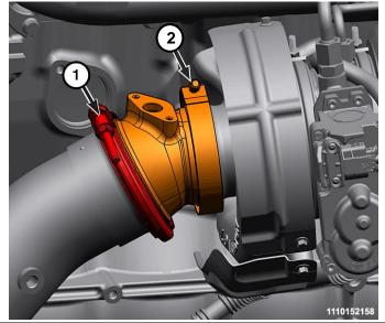
24. Remove the right side turbocharger to exhaust manifold nuts (1).
