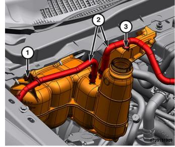
25. Install the right CAC tube (2), and tighten clamp nuts (1, 3) to **11 Nm (8 ft-lbs)**.
