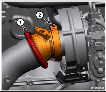
10. Install the exhaust isolator (2) and the transmission oil cooler line bracket to the transmission and tighten the bolts (1, 3) to 24 Nm (18 ft-lbs).
