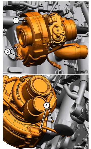
9. Using a NEW gasket (68437471AA) at the rear (1) of the exhaust outlet connector elbow, correctly align the elbow and pipe, and then tighten the forward band clamp (2) to 17 Nm (13 ft-lbs), and the rear clamp (1) to 61 Nm (45 ft-lbs).
