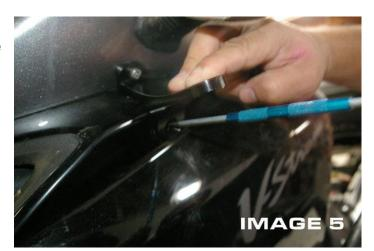
**Step 4:** While gently pressing down on the bracket, use a scribe to mark fairing where lower mounting point is located.
