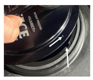
Model Years 2004-2007 6.0L Powerstroke: Orient the SureFlo sending unit to where the indented mark on the cap lines up with the dot on the tank as shown at right.
