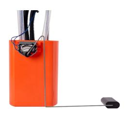
**STEP 12:** Install the new SureFlo sending unit into the tank as shown at right. See the application specific instructions below for proper clocking of your sending unit. Reinstall the locking ring.
