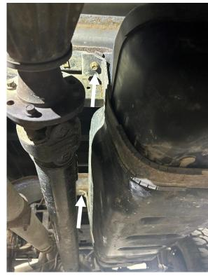
**STEP 6:** Lower the tank five to six inches and disconnect the electrical harness connector for the sending unit. Using a 3/8" quick disconnect tool, remove the fuel feed connector (blue quick connect fitting shown at right). Using a 5/16" quick disconnect tool, remove the fuel return connector (white quick connect fitting shown at right).
