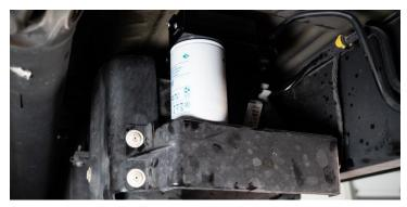
**STEP 14:** Prime the fuel system by cycling the ignition to the on position and waiting five seconds. Repeat this process two to three times, then start the vehicle. Check for leaks.
