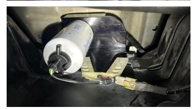
**STEP 13 (SHORT BED VEHICLES ONLY):** Install the guard back onto the tank using the three plastic clips removed in step 3. With the center section of the clip still pulled out, install the clips into the mounting holes. Push the center section into the clip to lock them in place.
