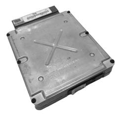
STEP 11 - Replace the bolts or nuts removed earlier holding the PCM in place.
