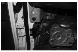
**STEP 4 -** Remove the plastic cap to expose the terminal.
