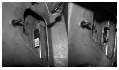
**STEP 5 -** With the provided Scotch-Brite pad clean the rubberized protective coating off of the terminal contacts. Both sides of the terminal need to be cleaned. It is important that the contacts are sufficiently clean to avoid any connection issues.
