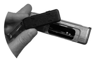
**STEP 6 -** With the provided Scotch-Brite pad clean the rubberized protective coating off of the terminal contacts. Both sides of the terminal need to be cleaned. It is important that the contacts are sufficiently clean to avoid any connection issues.
