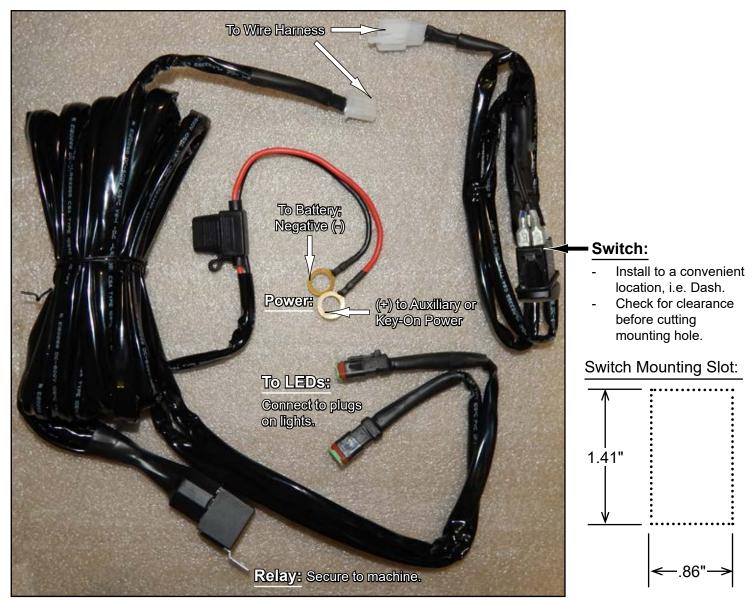
Ensure that all wires, relays, etc., are routed away from any moving or hot parts. Secure with wire ties.
