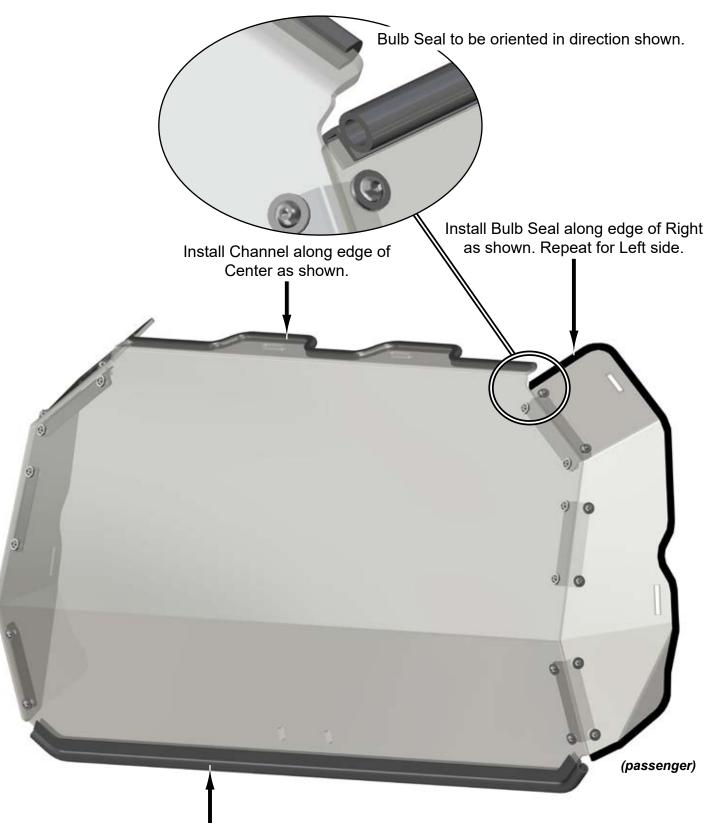
Install Seal along lower edge of Center as shown.
