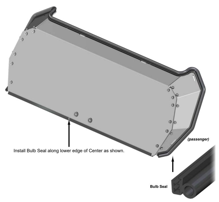
Install Bulb Seal along outer edges of assembly as shown.
