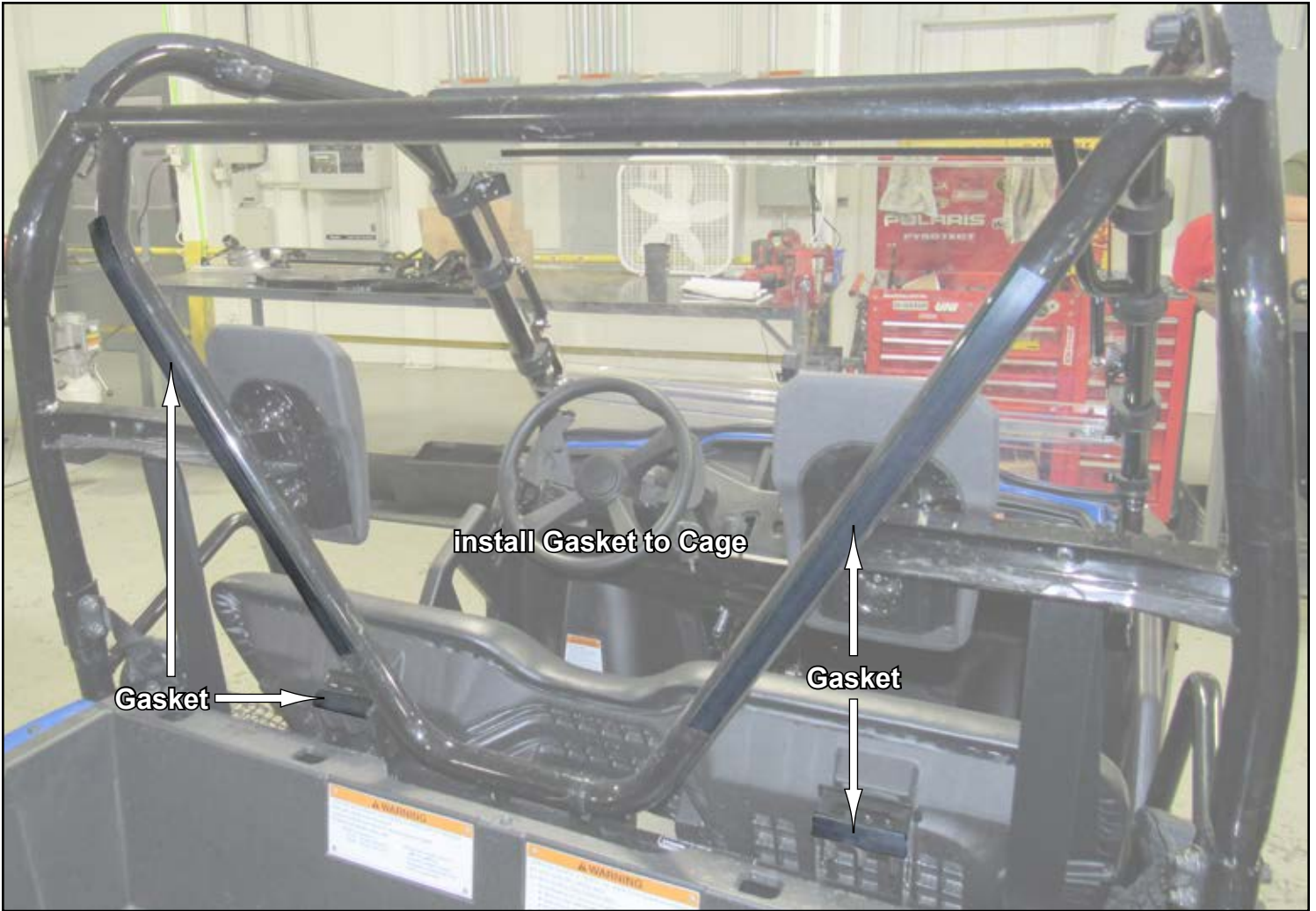
install Gasket to Brackets in location shown
