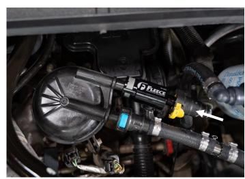
**STEP 10:** Prime the fuel system by cycling the ignition to the on position without starting the vehicle. Verify no leaks are present. Start the vehicle and check for leaks.
