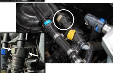
**STEP 4:** Cut the fuel injector return line just below the bottom of the fitting (see line in image) using hose cutters or diagonal cutters.
