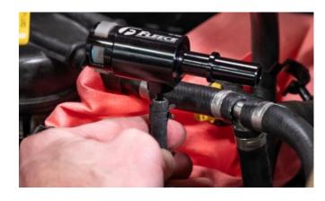
**STEP 7:** Using pliers, move hose clamp upward and position the hose clamp over the barb fitting.
