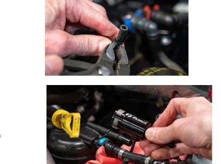
**STEP 6: Lubricate** the hose barb fitting with clean fuel to ease installation into the injector return hose. Press the barb fitting into the hose until both barbs are fully covered by the hose.
