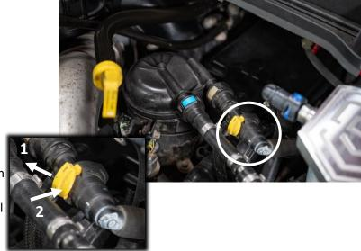
**STEP 3:** Disconnect the fuel feed fitting (gray plastic release buttons shown) from the filter assembly. Push the fitting towards the filter to release tension on the retainer. Squeeze both of the gray buttons and pull the fitting away from the filter to remove.
