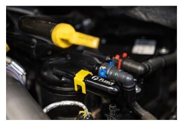
If the fitting requires maintenance, a service kit is available, Fleece Performance P/N: <u>FPE-FMC-FF-RLK-1724-SER</u>. The kit includes replacement O-rings and locking tabs.
