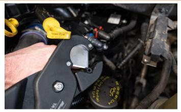
**STEP 5:** Using pliers, install the included hose clamp onto the injector return hose so that it is approximately one inch from the end of the hose to allow for the barb fitting to be easily installed.
