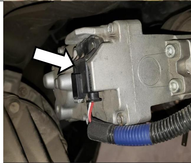
Lastly, route the harness with the black 4-pin connector down the firewall, along the frame rail to the exhaust brake actuator. Connect to the actuator and secure the harness along the frame.
