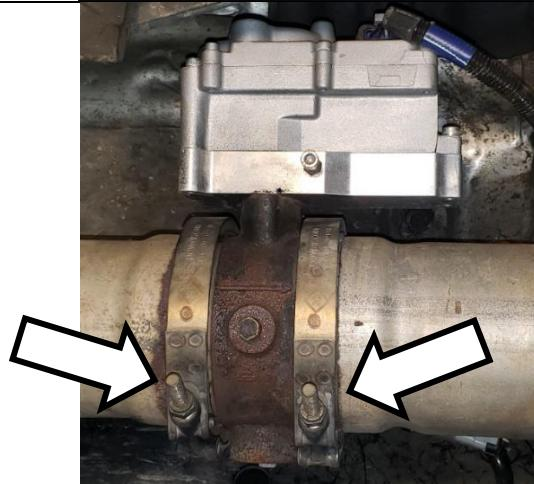
Weld the front adapter to the exhaust pipe. This weld must completely seal the exhaust system as it must retain pressure.
