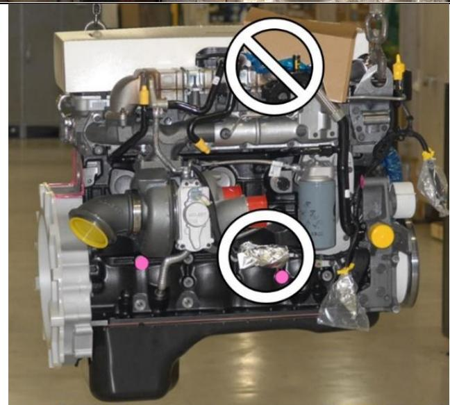
Route the electrical harness grey 12-pin connector up to the top rear of the passenger side battery.
