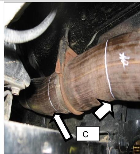
Cut out the marked pipe section using a reciprocating saw or cutting disk. Remove any burrs left on the edge of the pipe using a file or similar tool, then slide the pipe adapters onto the two cut ends of the pipe.
