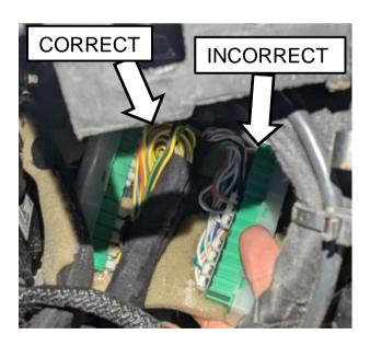
Locate the factory turbocharger actuator electrical connector. This is the 4-pin black connector that used to be connected to the VGT. Connect the black connector of the harness for power and ground.
