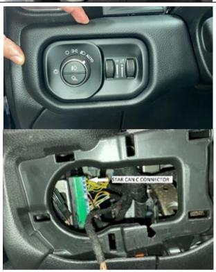
Plug the 2-pin connector from the BD harness into any open ports on the junction block connected to a bundle of yellow wires with a green housing.
