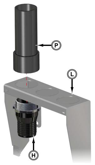
remove any remaining slack by rotating Locknut up until tight against Bracket (L)
