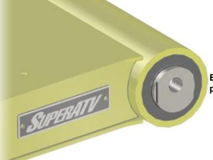
Bearing in this position provides positive camber (tire out at top)
