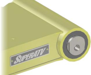
Bearing in this position provides negative camber (tire in at top)
