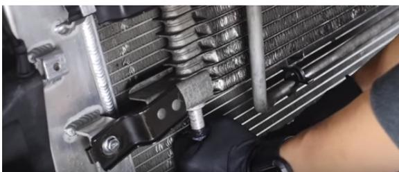
9. Separate the transmission cooler brackets from both sides of the radiator. Then, remove the transmission cooler. (2x 10mm bolts)
