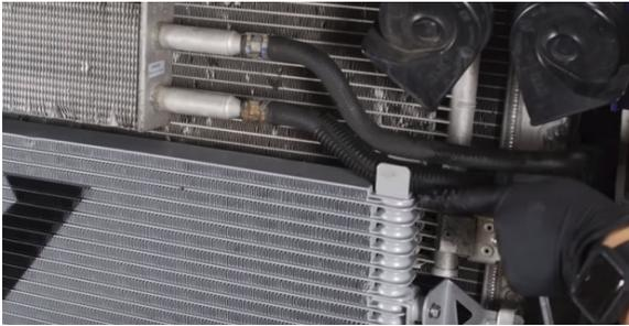
15. Install the provided hose to the radiator and transmission cooler ports. Be sure to slide a clamp on each end before attaching them to the ports. (2x worm gear clamps)
