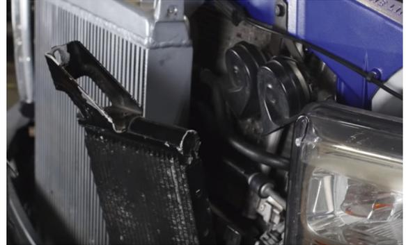
2. Loosen the clamps on the coupler between the intercooler and hot-side pipe. Slide the coupler off the intercooler end tank. (2x t-bolt clamps)
