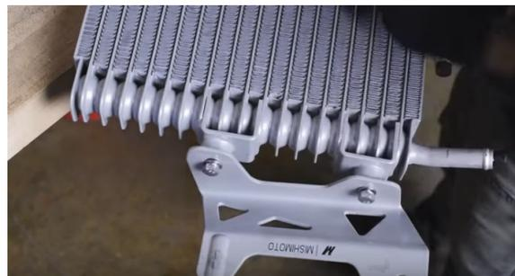
12. Install the Mishimoto transmission cooler. Position the top of the cooler brackets underneath the two tabs on the radiator. Secure the brackets with the provided hardware. If you have a Mishimoto rad installed, place the spacer behind the bracket.
