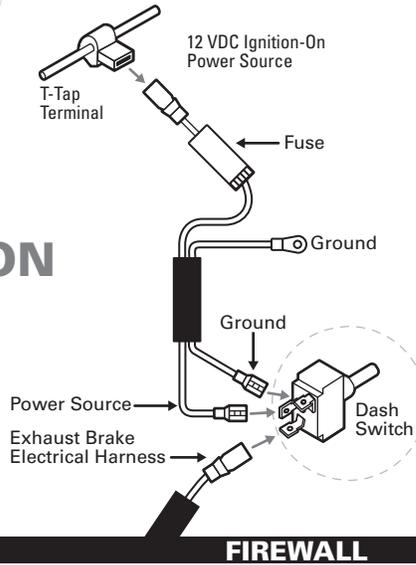
EXHAUST BRAKE CONNECTIONS WITH OPTIONAL SWITCH-PAC
