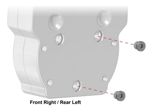
install into each Gear Box Torque to 10 ft/lbs
