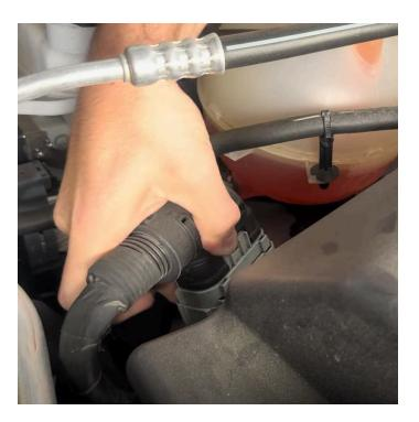
Disconnect the MAF by unlocking the tab and then depressing the lever as you pull it off.
