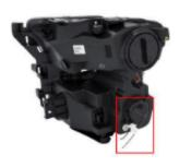
The two wires located at the bottom of the new AnzoUSA headlight will operate the switchback function.
