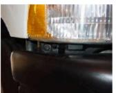
Step 5: Remove the second 10mm screw under the corner light.
