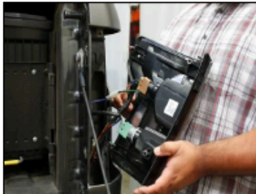
Connect both factory connections and resistor to Anzo USA tail light.
