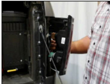
Guide tail light locating pins into fender well. Install two 8mm bolts for tail light.
