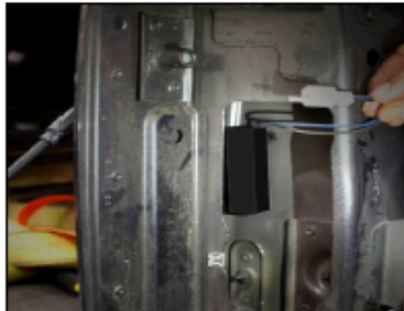
Clean surface area in fender well with mild soap or rubbing alcohol to remove any dirt and grime.
