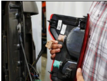
Disconnect both connections from factory tail light.
