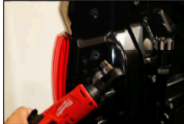
Lower tailgate then remove top and bottom 10 mm bolt.
