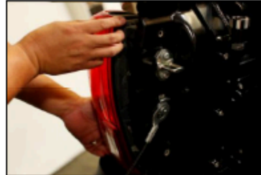
Pull tail lights towards back of vehicle to remove.
