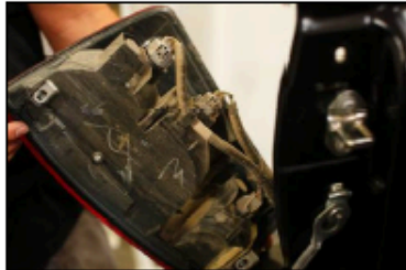
Disconnect three connections on factory tail light and remove.
