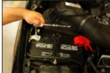
Open hood and disconnect negative battery terminal
