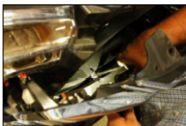
Tilt top of grill forward to reveal bottom grill clips. Use flat head screwdriver to push clip down.
