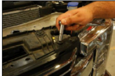
Remove eight 8mm bolts from top of radiator grill
