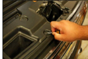
Remove 13 body panel clips from radiator shroud
