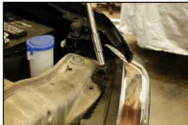
Remove top 10mm headlight bolt
