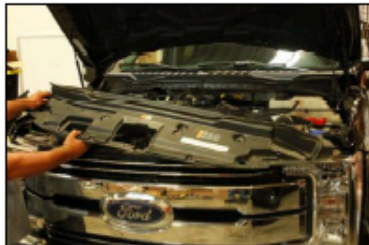
Remove radiator shroud and set aside
