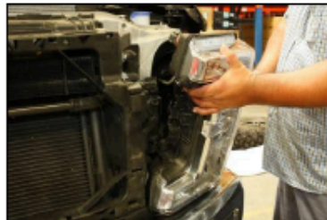
Slide headlight forward then up to remove headlight. Disconnect all connections from factory headlight
