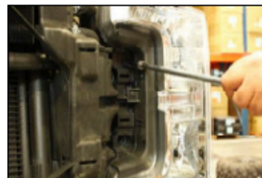
Remove two 10mm inner headlight bolts
