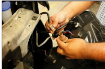
Connect factory connections to new Anzo USA headlight
