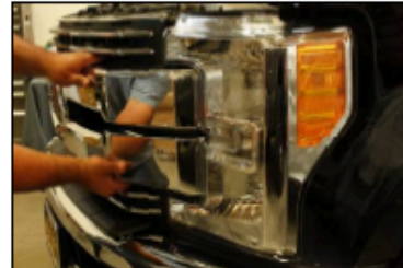
Grab center outside of grill and pull forward to detach grill from headlight on both sides.
