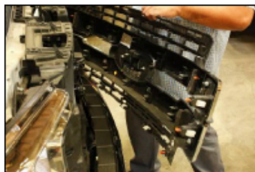
Detach 4 clips remove grill and set aside
